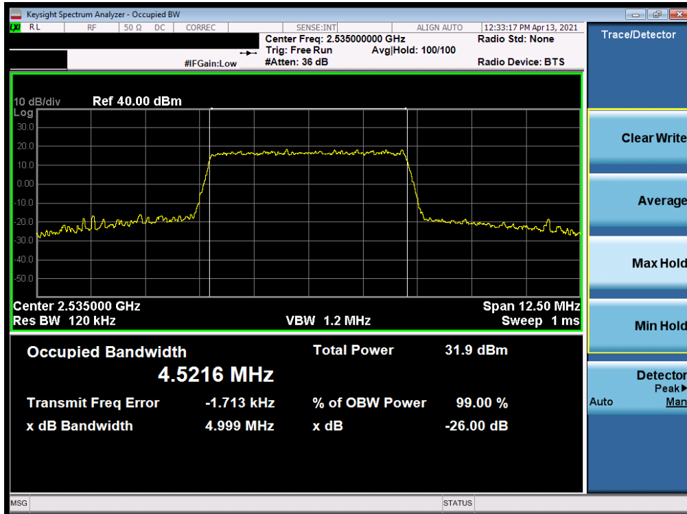
Plot 7-12. Occupied Bandwidth Plot (LTE Band 7 - 5MHz 16-QAM - Full RB)
