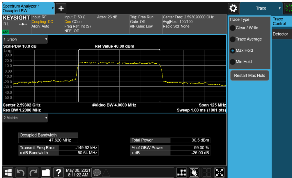
Plot 7-72. Occupied Bandwidth Plot (NR Band n41 - 50MHz QPSK - Full RB)
