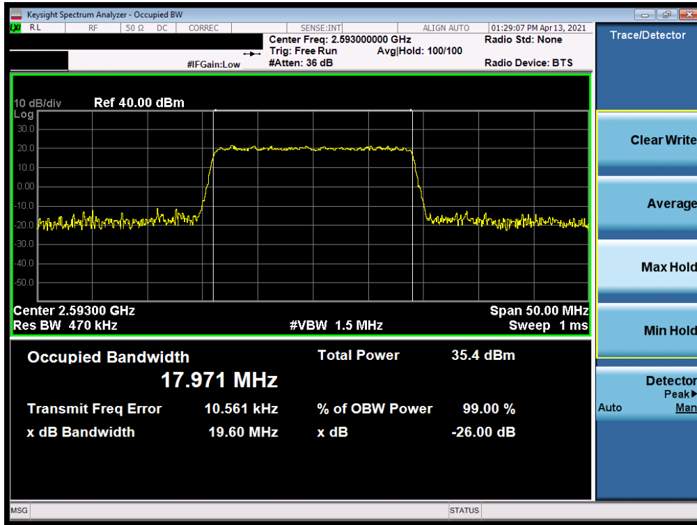
Plot 7-13. Occupied Bandwidth Plot (LTE Band 41(PC2) - 20MHz QPSK - Full RB)
