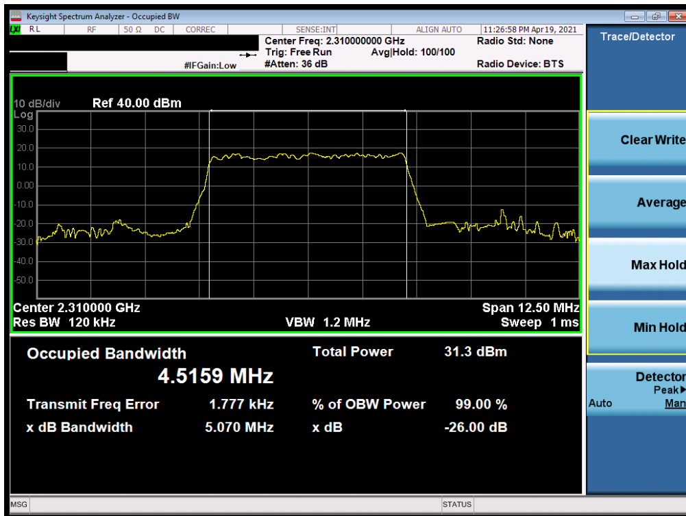
Plot 7-32. Occupied Bandwidth Plot (NR Band n30 - 5MHz \pi/2 BPSK - Full RB)
