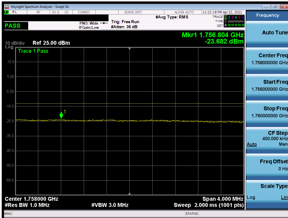
Plot 7-217. Upper Extended Band Edge Plot (LTE Band 4 - 15MHz QPSK – Full RB)
