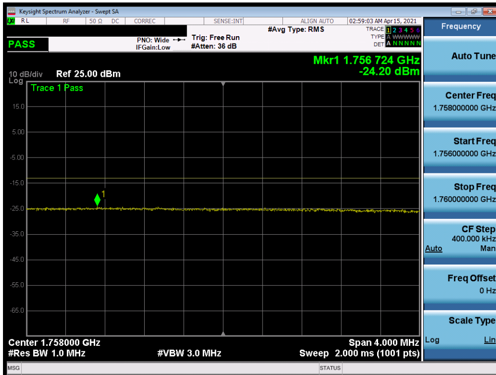
Plot 7-211. Upper Extended Band Edge Plot (LTE Band 4 - 20MHz QPSK – Full RB)
