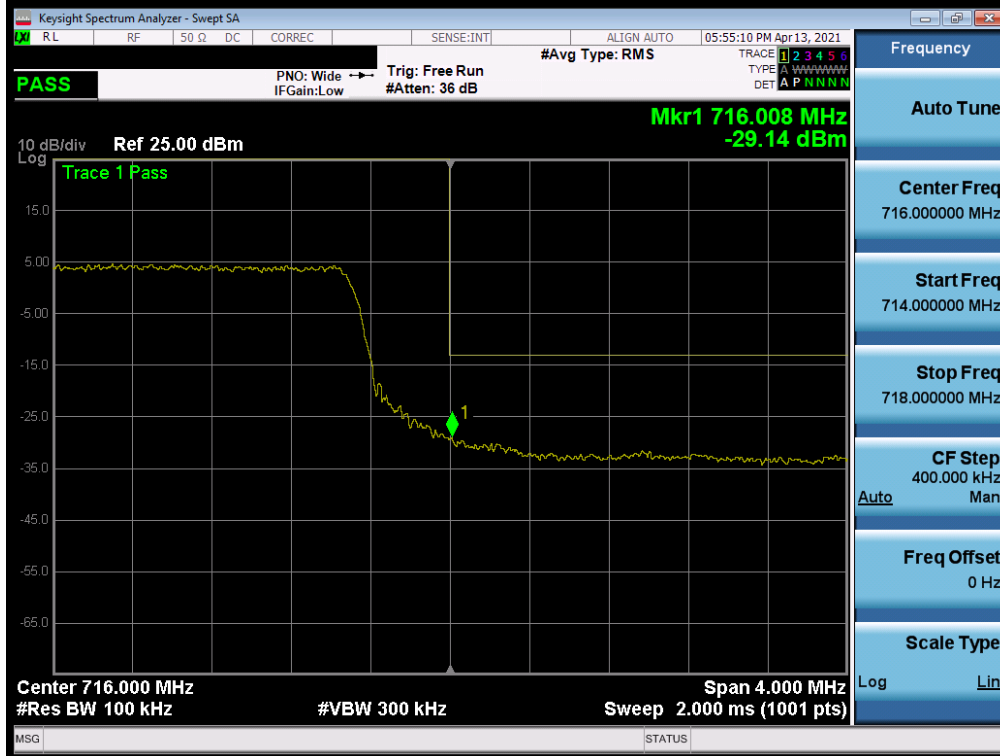
Plot 7-175. Upper Band Edge Plot (LTE Band 12 - 10MHz QPSK – Full RB)
