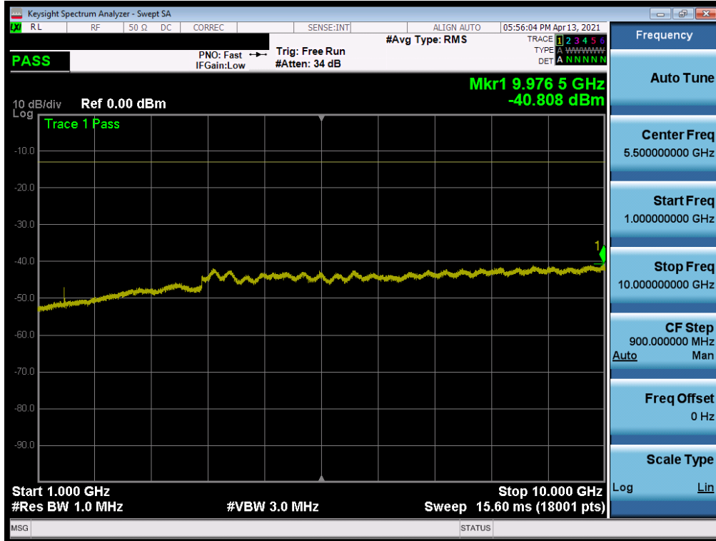
Plot 7-108. Conducted Spurious Plot (LTE Band 12 - 10MHz QPSK - RB Size 1, RB Offset 0 - High Channel)
