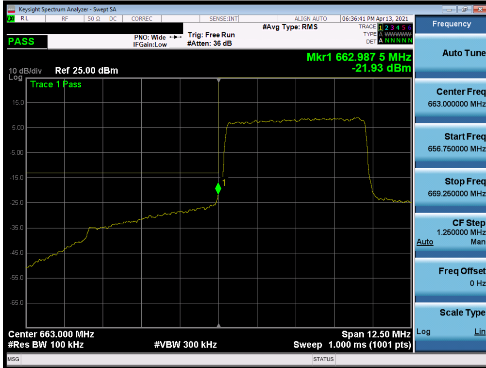
Plot 7-172. Lower Band Edge Plot (LTE Band 71 - 5MHz QPSK – Full RB)
