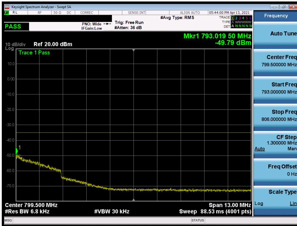
Plot 7-185. Upper Emission Mask Plot (LTE Band 13 - 10MHz QPSK – Full RB)
