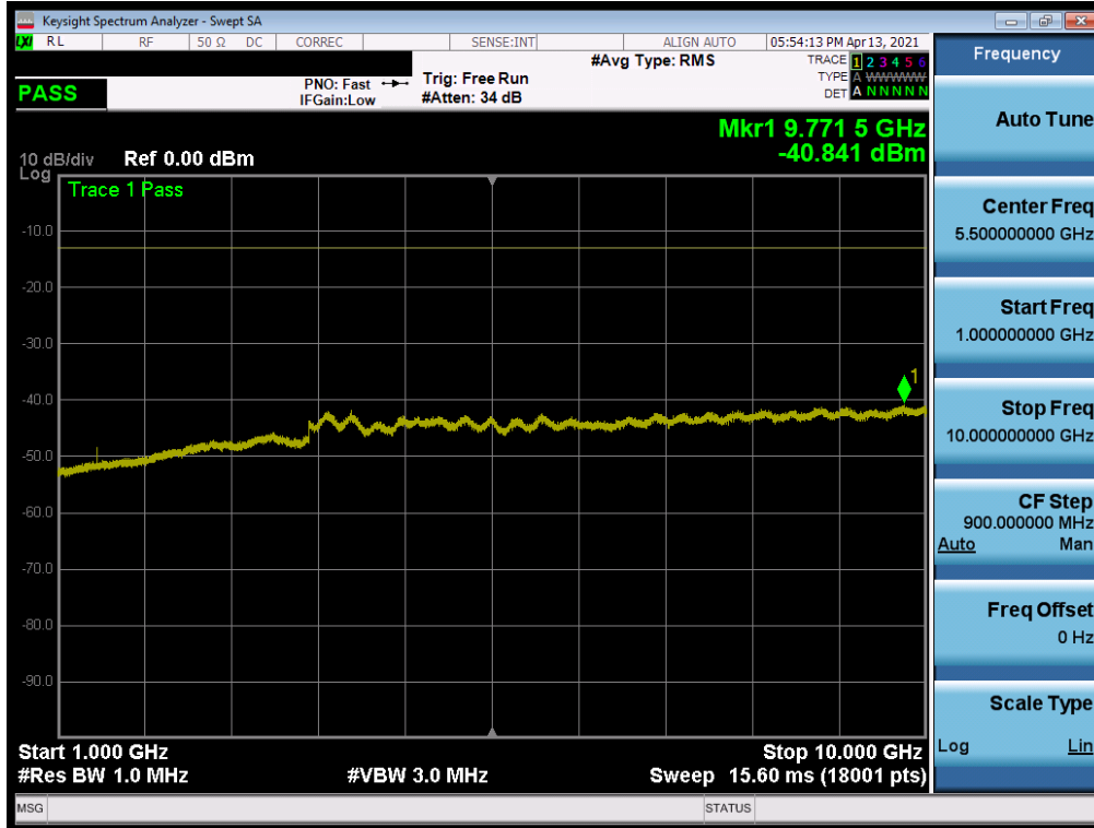
Plot 7-102. Conducted Spurious Plot (LTE Band 12 - 10MHz QPSK - RB Size 1, RB Offset 0 - Low Channel)
