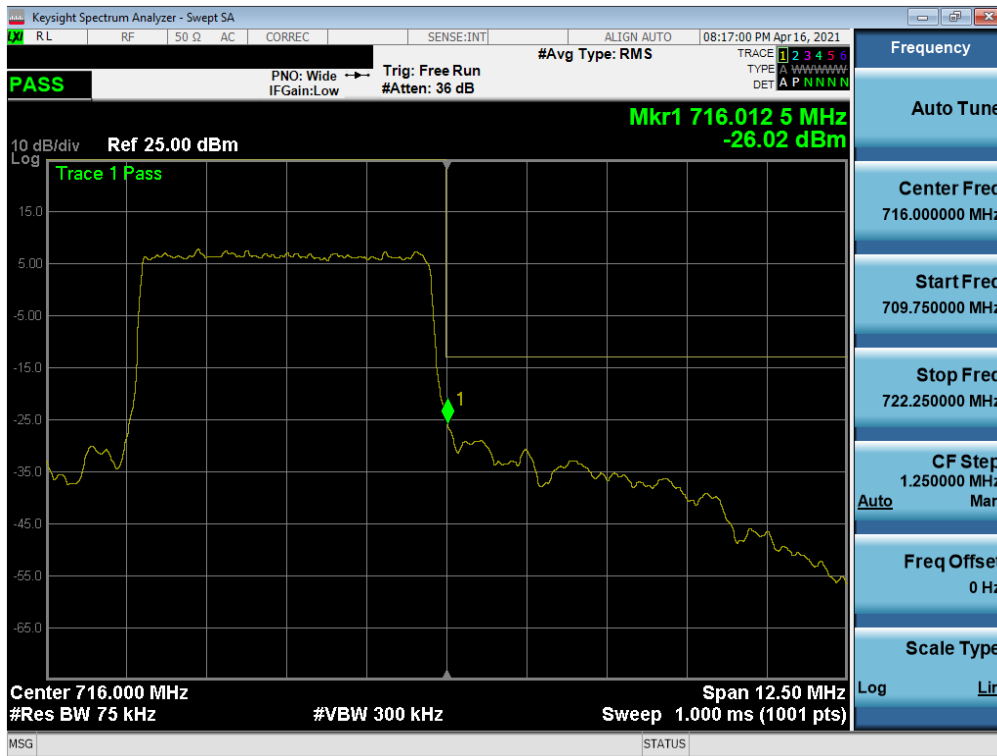
Plot 7-203. Upper Band Edge Plot (NR Band n12 – 5.0MHz - Full RB)
