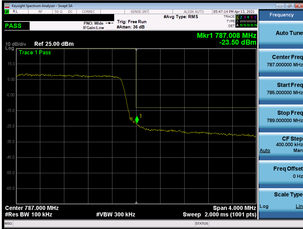
Plot 7-188. Upper Band Edge Plot (LTE Band 13 - 5MHz QPSK – Full RB)
