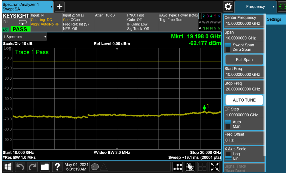
Plot 7-159. Conducted Spurious Plot (NR Band n66 - 40.0MHz - 1 RB - Low Channel)
