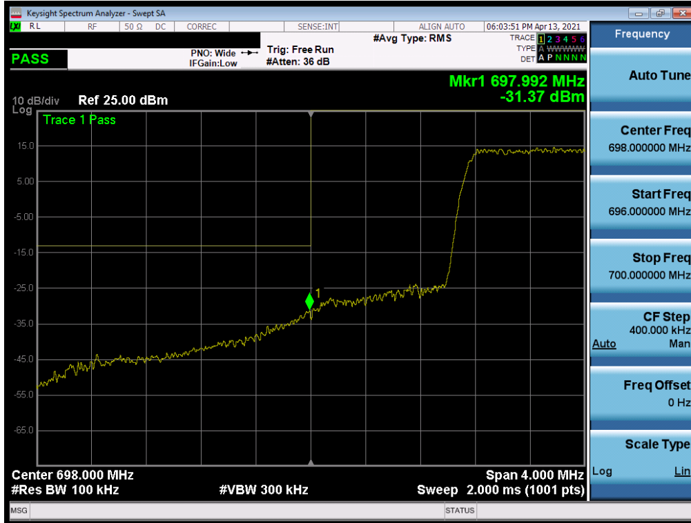
Plot 7-180. Lower Band Edge Plot (LTE Band 12 – 1.4MHz QPSK – Full RB)
