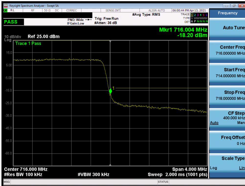
Plot 7-179. Upper Band Edge Plot (LTE Band 12 - 3MHz QPSK – Full RB)
