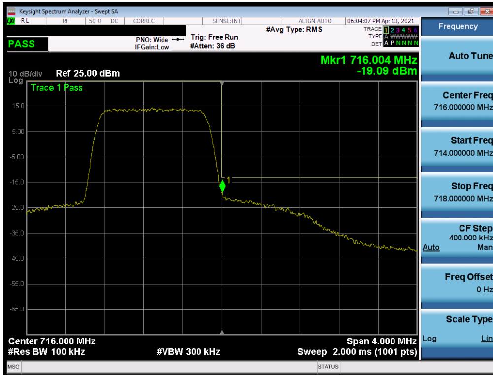
Plot 7-181. Upper Band Edge Plot (LTE Band 12 – 1.4MHz QPSK – Full RB)
