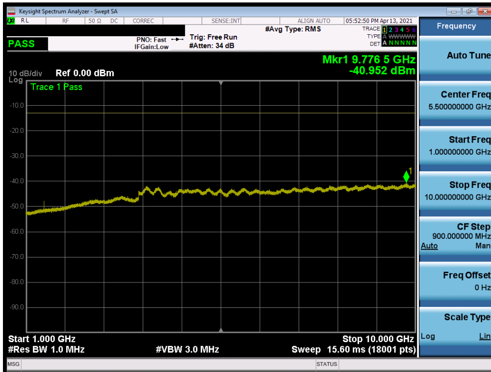
Plot 7-105. Conducted Spurious Plot (LTE Band 12 - 10MHz QPSK - RB Size 1, RB Offset 0 - Mid Channel)
