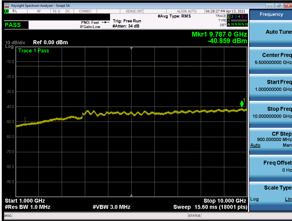
Plot 7-99. Conducted Spurious Plot (LTE Band 71 - 20MHz QPSK - RB Size 1, RB Offset 0 - High Channel)
