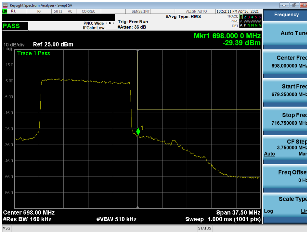
Plot 7-193. Upper Band Edge Plot (NR Band n71 – 15.0MHz - Full RB)
