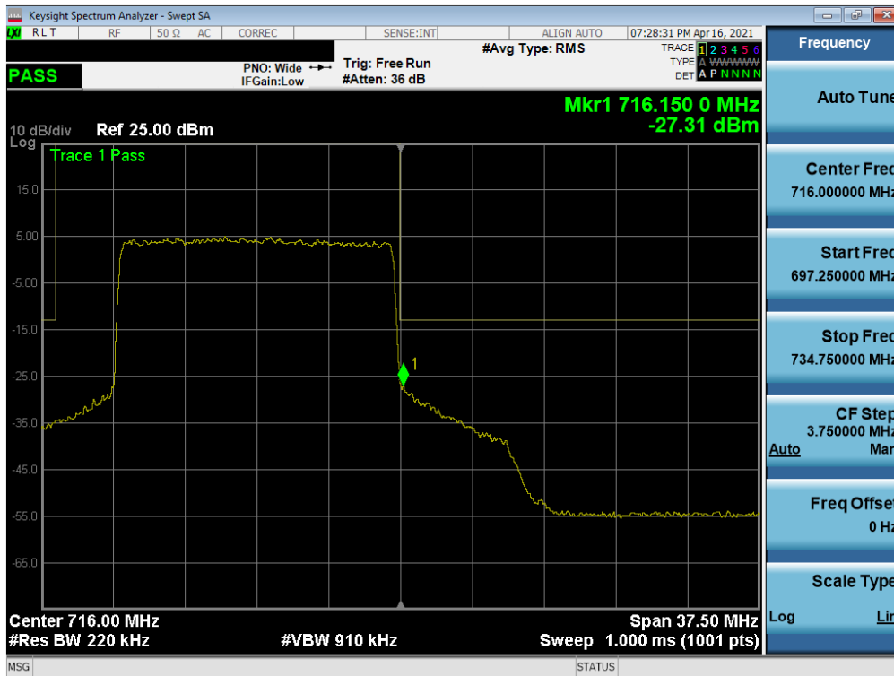
Plot 7-199. Upper Band Edge Plot (NR Band n12 – 15.0MHz - Full RB)
