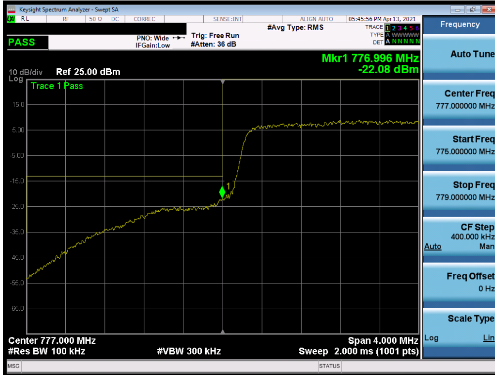
Plot 7-186. Lower Band Edge Plot (LTE Band 13 - 5MHz QPSK – Full RB)
