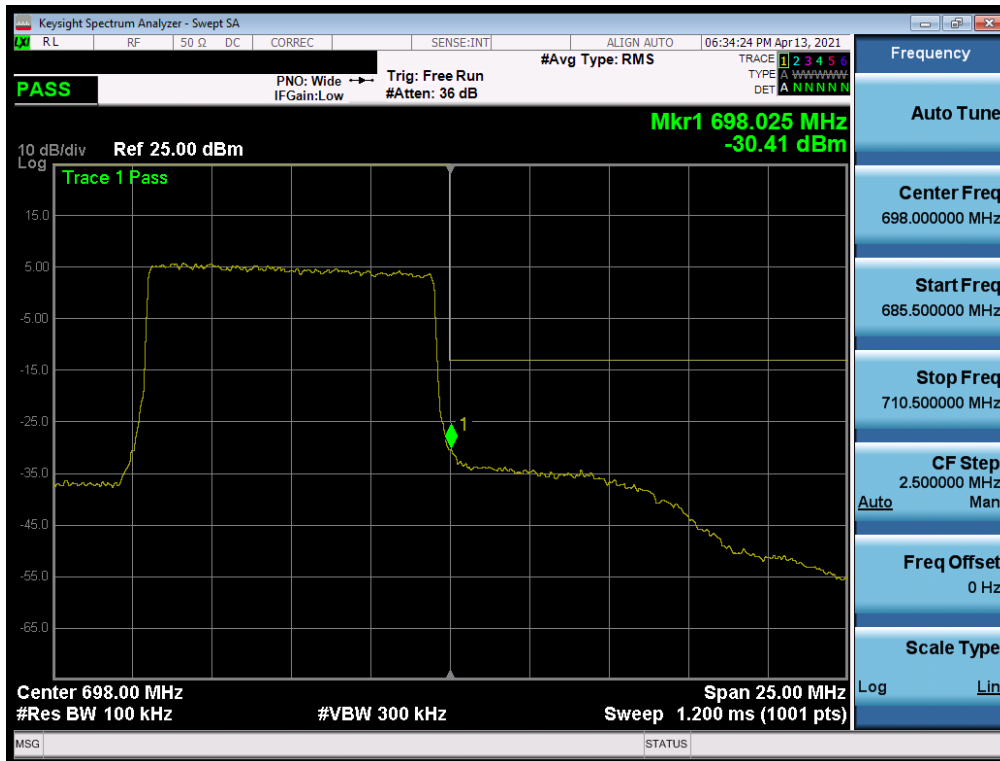
Plot 7-171. Upper Band Edge Plot (LTE Band 71 - 10MHz QPSK – Full RB)
