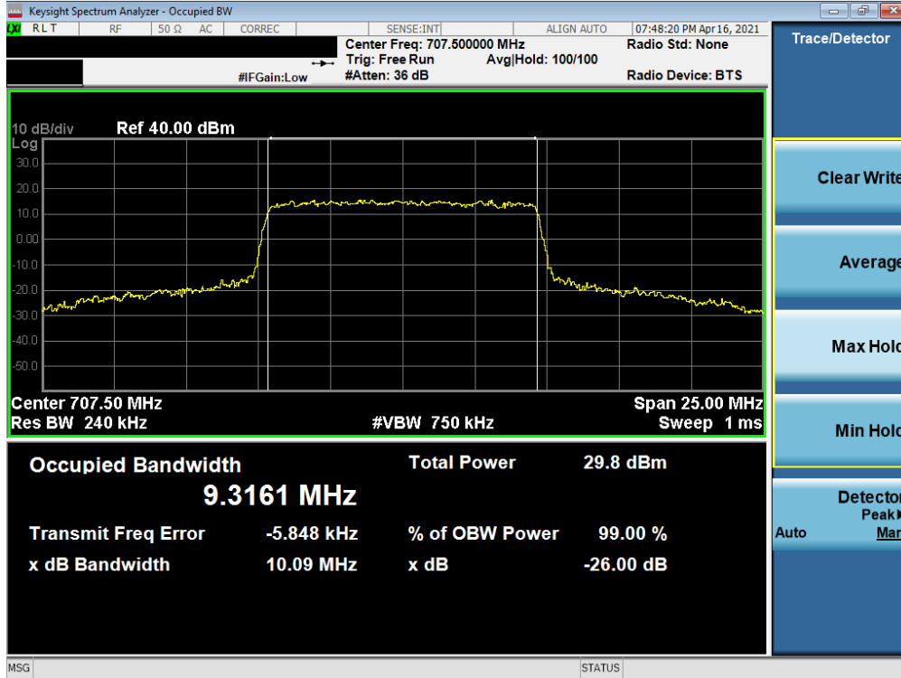
Plot 7-37. Occupied Bandwidth Plot (NR Band n12 - 10MHz CP-OFDM QPSK - Full RB)
