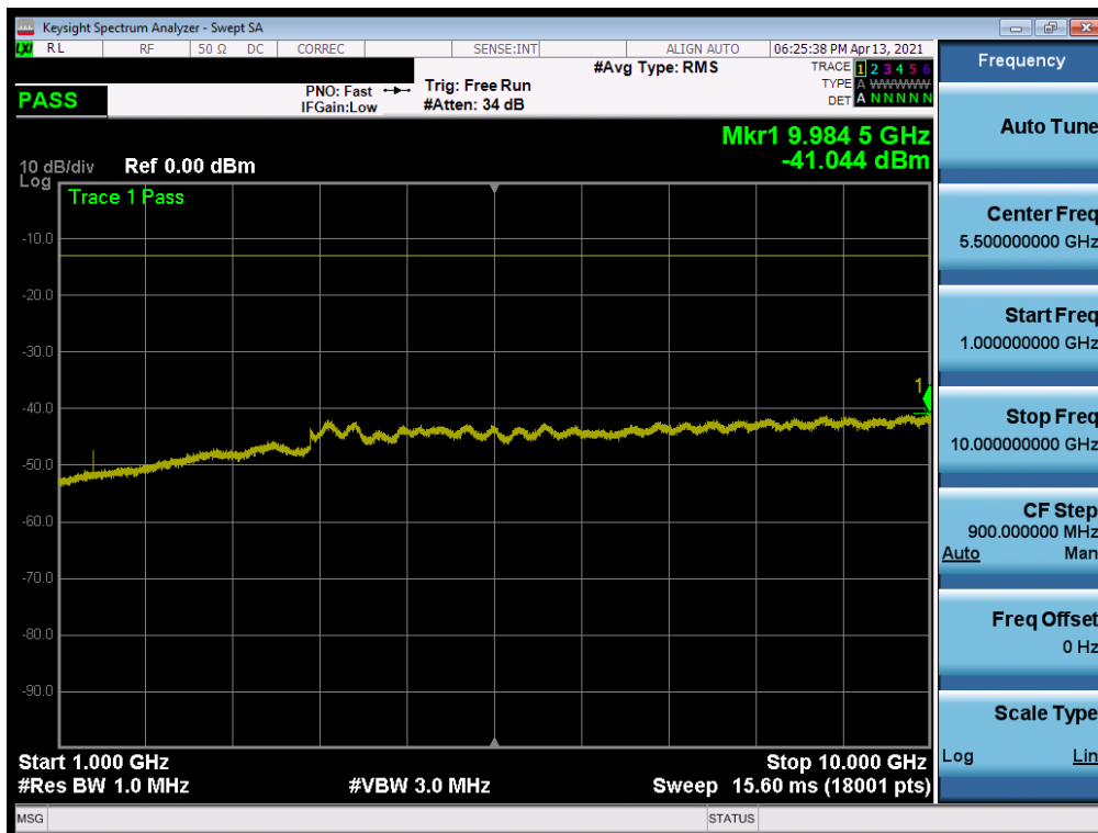
Plot 7-96. Conducted Spurious Plot (LTE Band 71 - 20MHz QPSK - RB Size 1, RB Offset 0 - Mid Channel)
