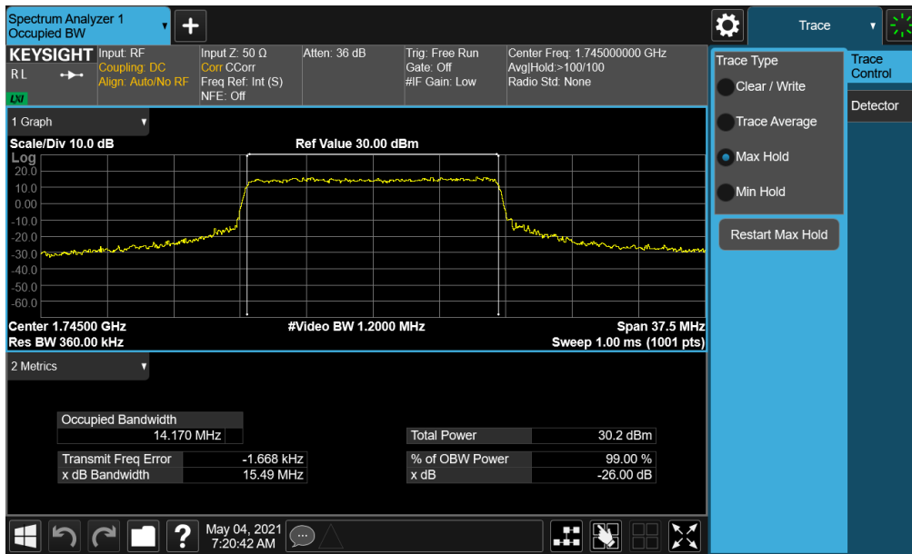
Plot 7-84. Occupied Bandwidth Plot (NR Band n66 - 15.0MHz CP-OFDM 16QAM - Full RB)
