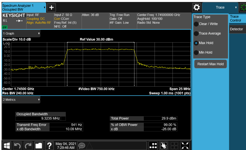
Plot 7-86. Occupied Bandwidth Plot (NR Band n66 - 10.0MHz CP-OFDM QPSK - Full RB)
