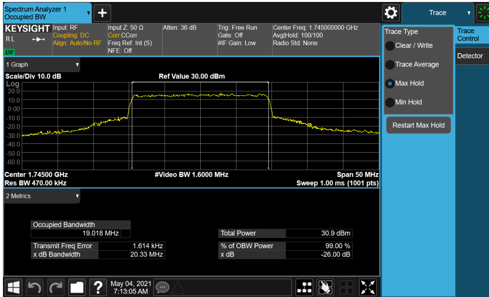
Plot 7-81. Occupied Bandwidth Plot (NR Band n66 - 20.0MHz CP-OFDM 16QAM - Full RB)
