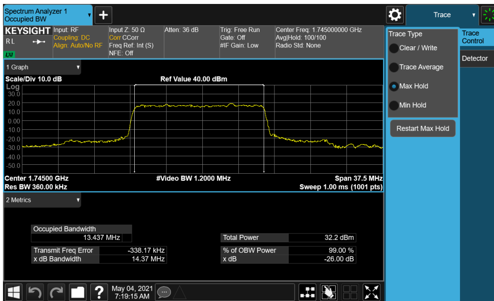
Plot 7-82. Occupied Bandwidth Plot (NR Band n66 - 15.0MHz DFT-s-OFDM BPSK - Full RB)
