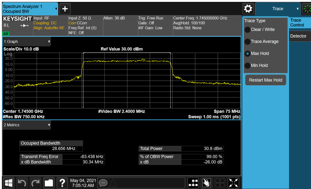
Plot 7-78. Occupied Bandwidth Plot (NR Band n66 - 30.0MHz CP-OFDM 16QAM - Full RB)
