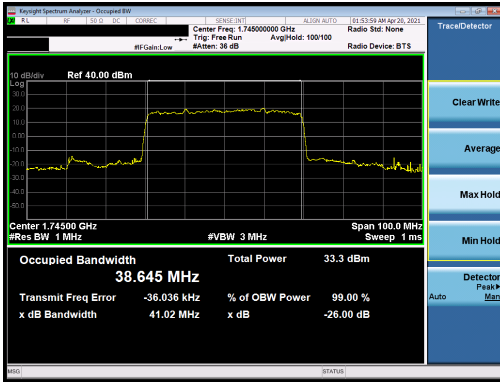
Plot 7-55. Occupied Bandwidth Plot (NR Band n66 - 40.0MHz DFT-s-OFDM BPSK - Full RB)
