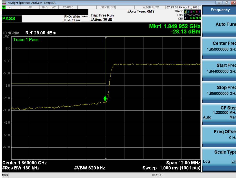
Plot 7-167. Lower Band Edge Plot (NR Band n25/2 - 15MHz QPSK – Full RB)
