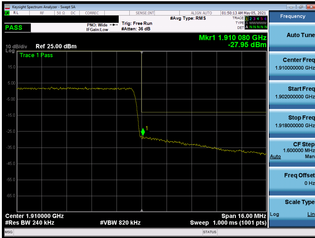
Plot 7-199. Upper Band Edge Plot (NR Band n2 – 20MHz QPSK – Full RB)
