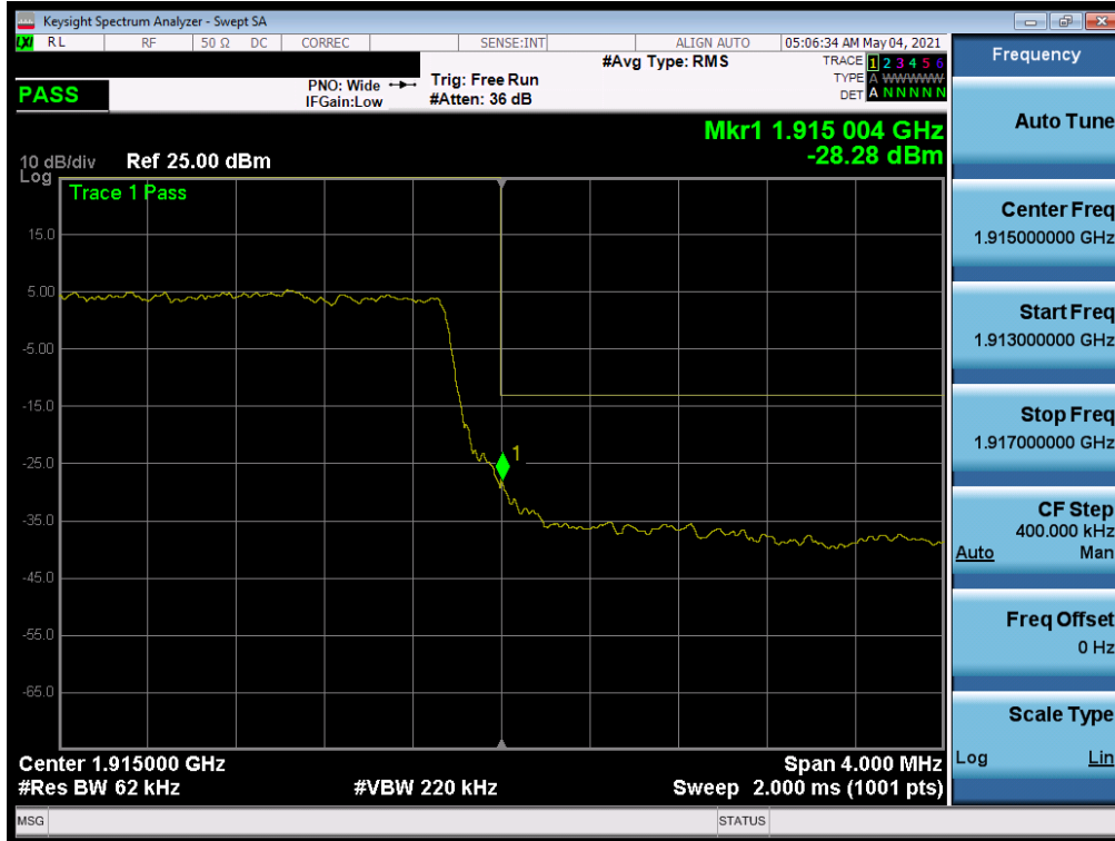
Plot 7-219. Upper Band Edge Plot (NR Band n25 – 5MHz QPSK – Full RB)
