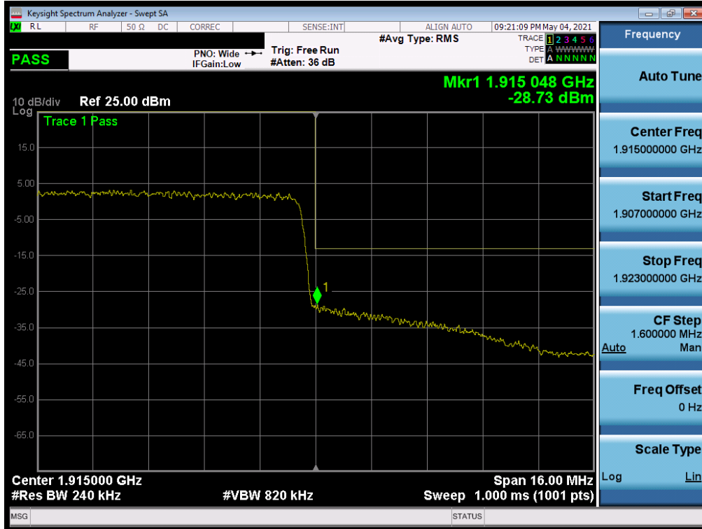
Plot 7-201. Upper Band Edge Plot (NR Band n25 – 20MHz QPSK – Full RB)
