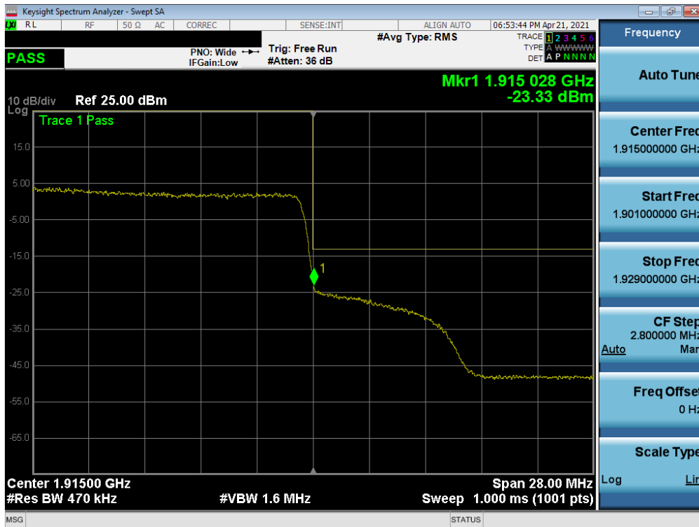
Plot 7-151. Upper Band Edge Plot (NR Band n25 - 40MHz QPSK – Full RB)
