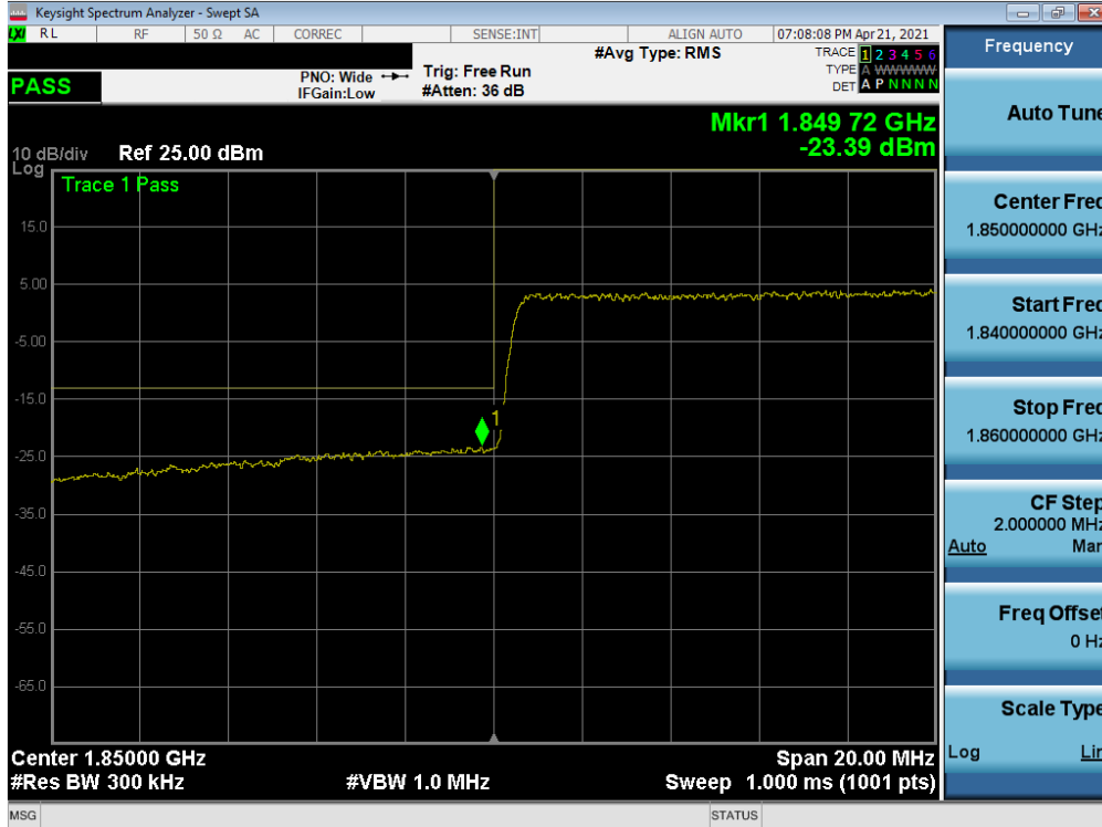
Plot 7-157. Lower Band Edge Plot (NR Band n25 - 25MHz QPSK – Full RB)
