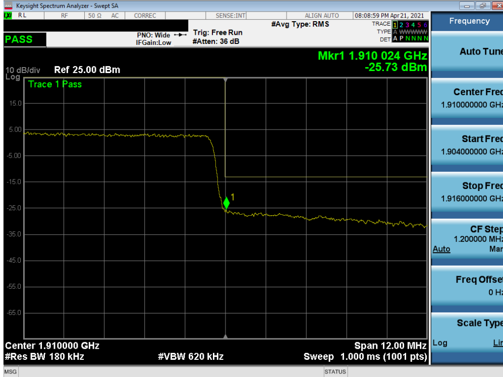
Plot 7-169. Upper Band Edge Plot (NR Band n2 - 15MHz QPSK – Full RB)
