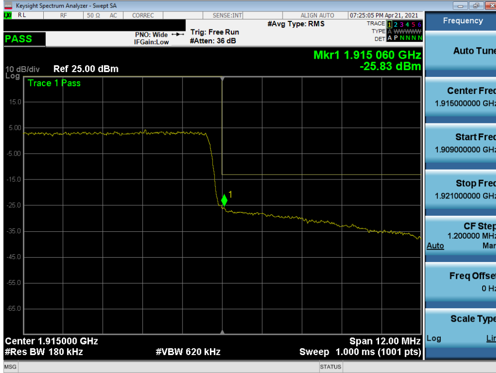
Plot 7-171. Upper Band Edge Plot (NR Band n25 - 15MHz QPSK – Full RB)
