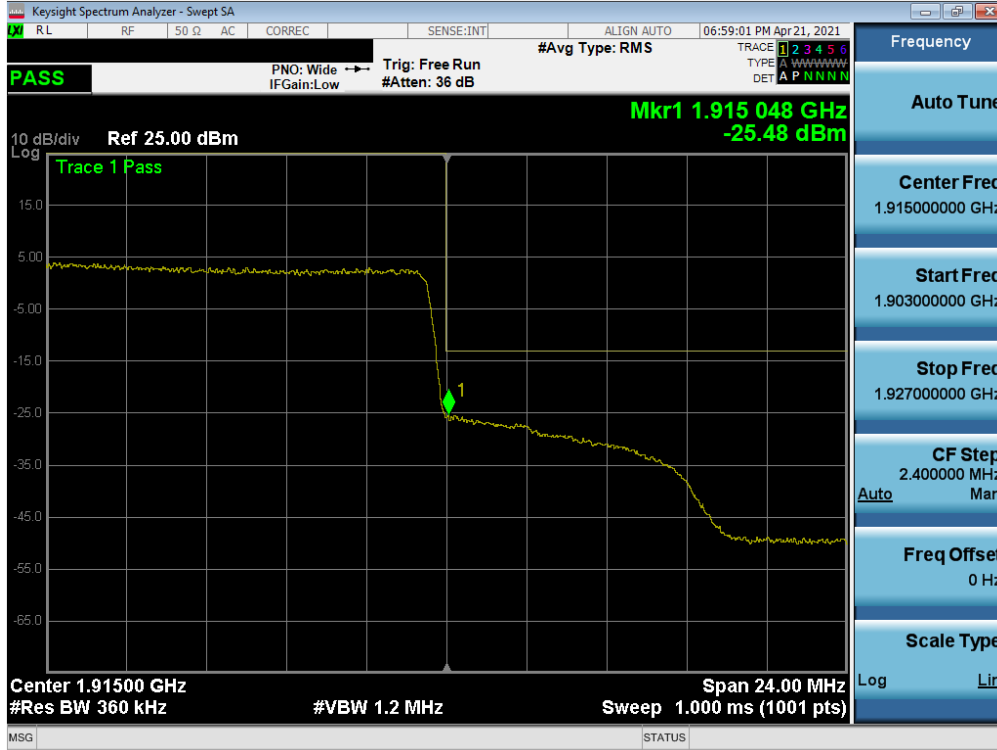
Plot 7-155. Upper Band Edge Plot (NR Band n25 - 30MHz QPSK – Full RB)
