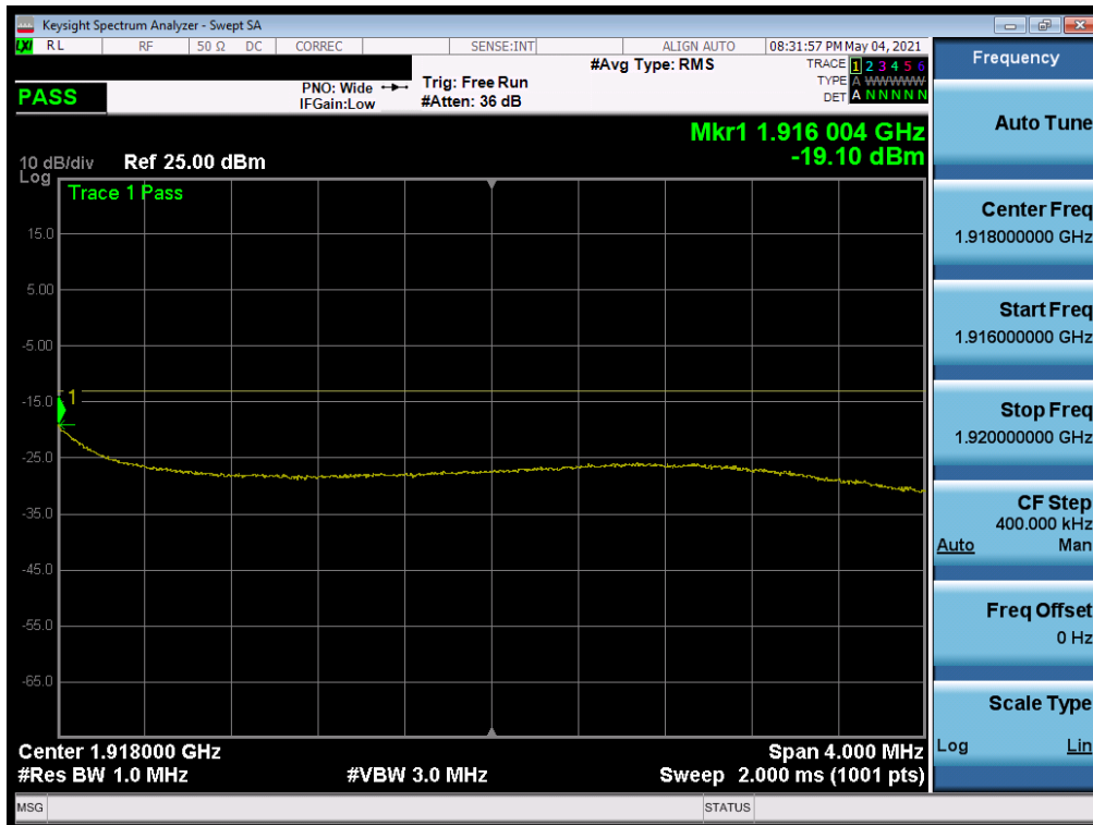
Plot 7-214. Extended Upper Band Edge Plot (NR Band n25 – 10MHz QPSK – Full RB)
