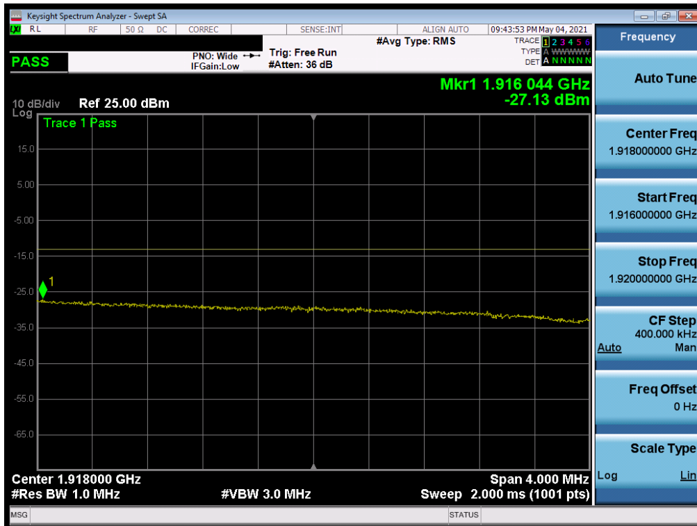
Plot 7-192. Extended Upper Band Edge Plot (NR Band n25 – 30MHz QPSK – Full RB)
