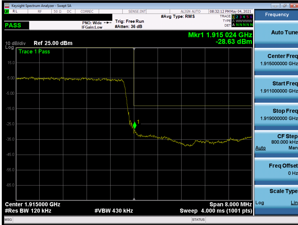
Plot 7-213. Upper Band Edge Plot (NR Band n25 – 10MHz QPSK – Full RB)
