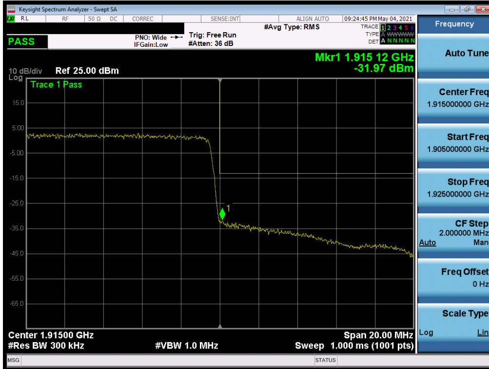
Plot 7-195. Upper Band Edge Plot (NR Band n25 – 25MHz QPSK – Full RB)
