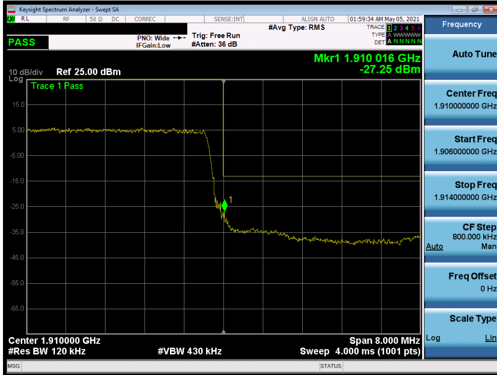
Plot 7-211. Upper Band Edge Plot (NR Band n2 – 10MHz QPSK – Full RB)
