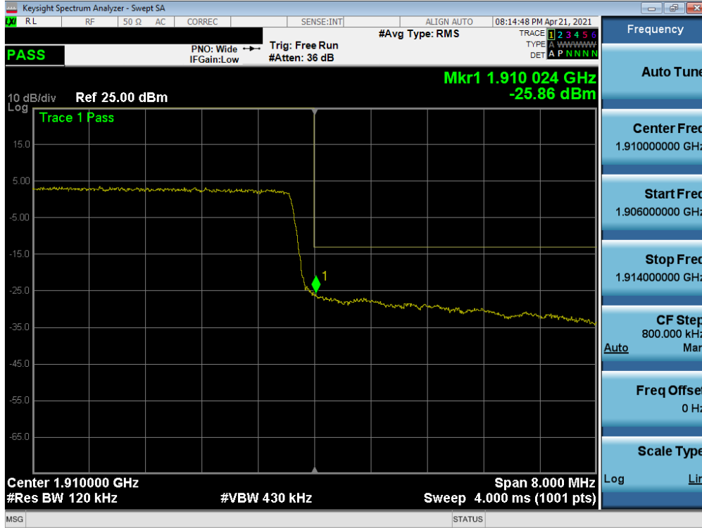
Plot 7-175. Upper Band Edge Plot (NR Band n2 - 10MHz QPSK – Full RB)
