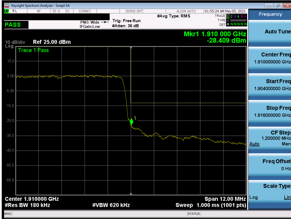
Plot 7-205. Upper Band Edge Plot (NR Band n2 – 15MHz QPSK – Full RB)
