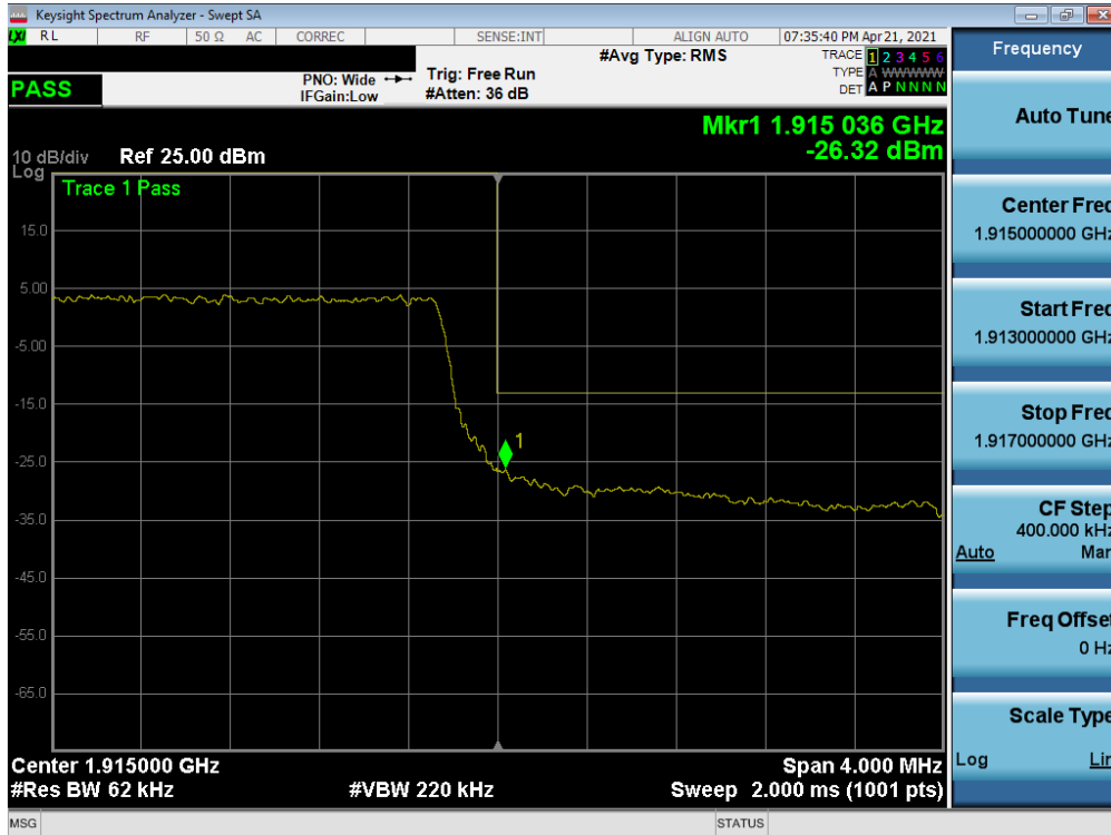
Plot 7-183. Upper Band Edge Plot (NR Band n25 – 5MHz QPSK – Full RB)
