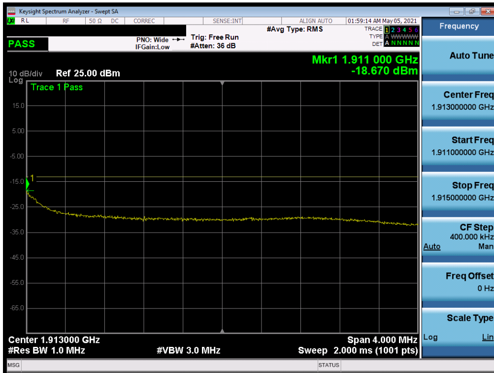
Plot 7-212. Extended Upper Band Edge Plot (NR Band n2 – 10MHz QPSK – Full RB 2)
