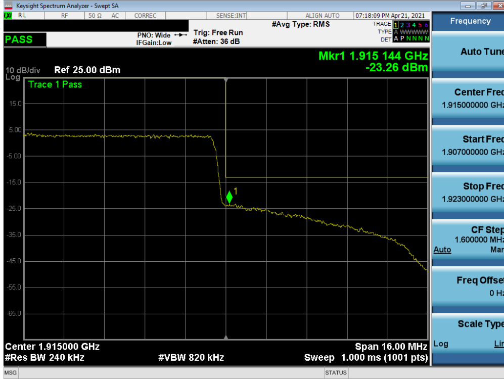
Plot 7-165. Upper Band Edge Plot (NR Band n25 - 20MHz QPSK – Full RB)
