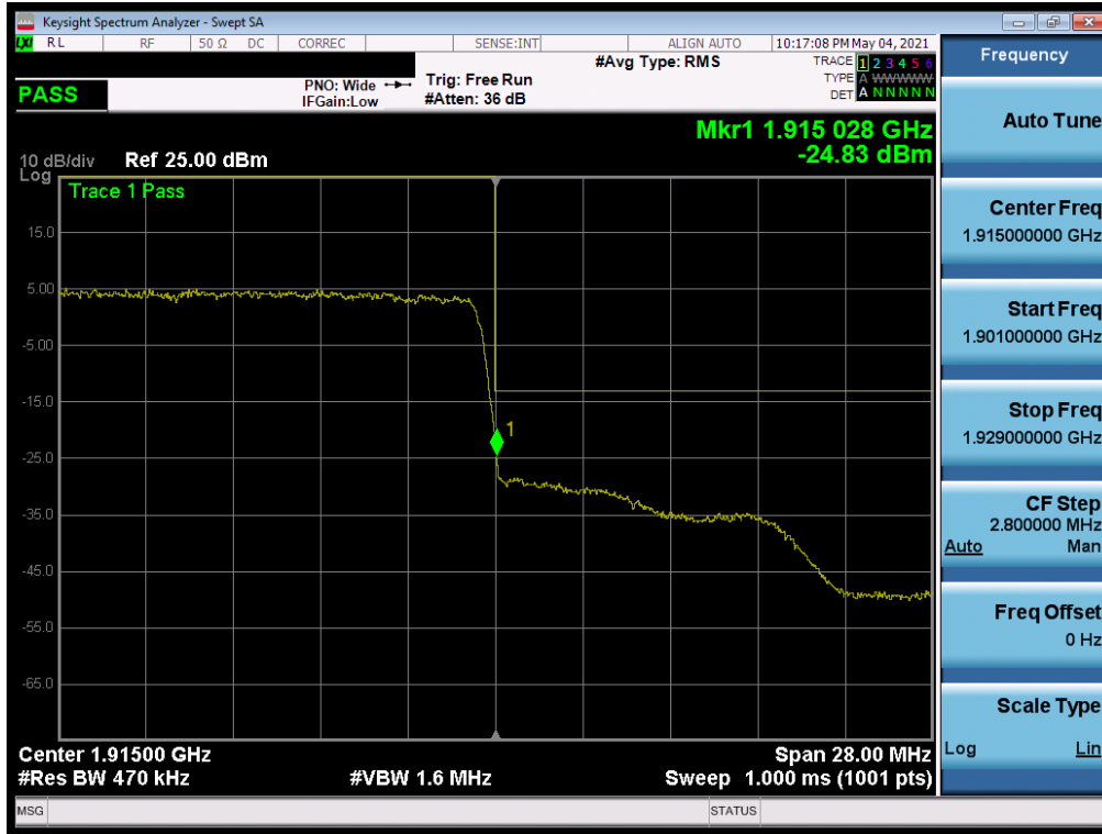
Plot 7-187. Upper Band Edge Plot (NR Band n25 – 40MHz QPSK – Full RB)
