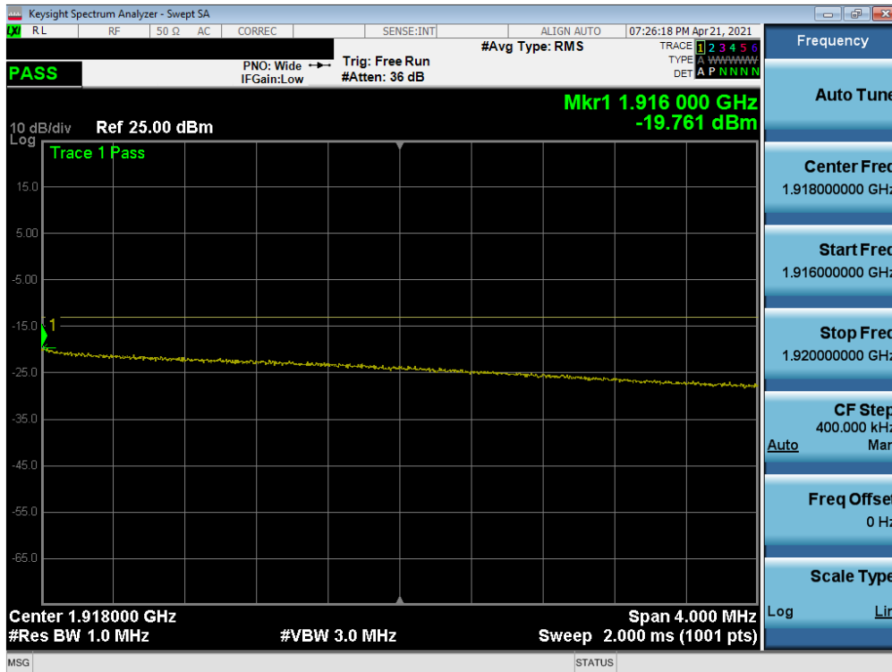
Plot 7-172. Extended Upper Band Edge Plot (NR Band n25 - 15MHz QPSK – Full RB)
