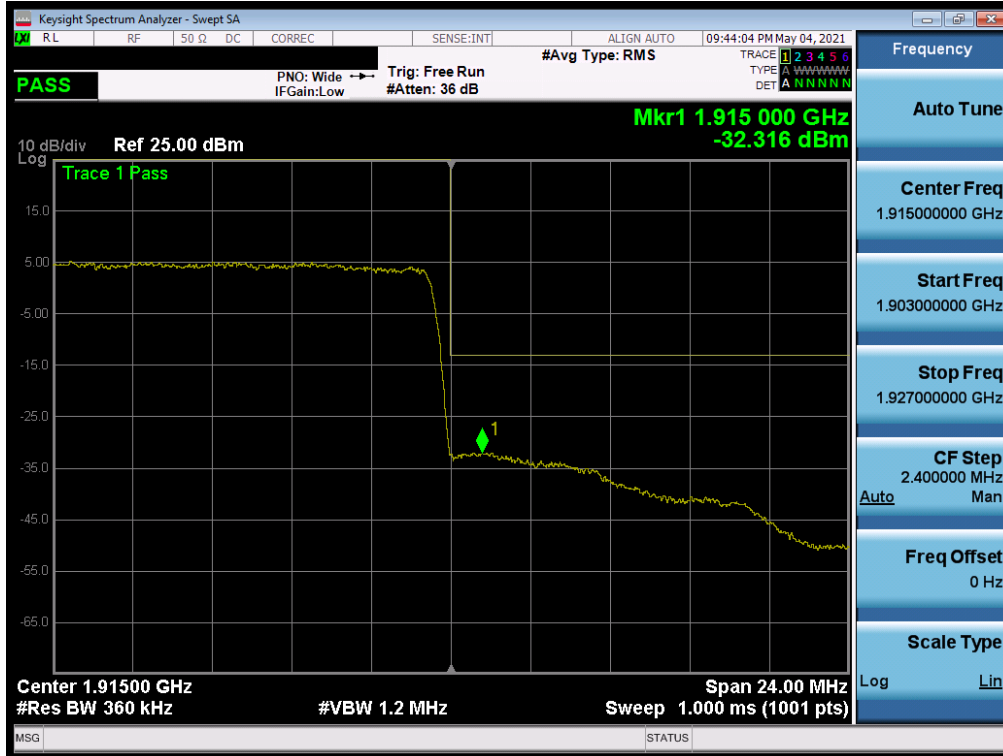
Plot 7-191. Upper Band Edge Plot (NR Band n25 – 30MHz QPSK – Full RB)
