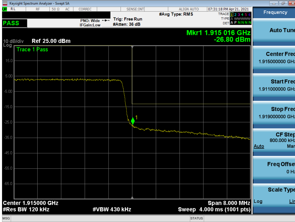
Plot 7-177. Upper Band Edge Plot (NR Band n25 - 10MHz QPSK – Full RB)
