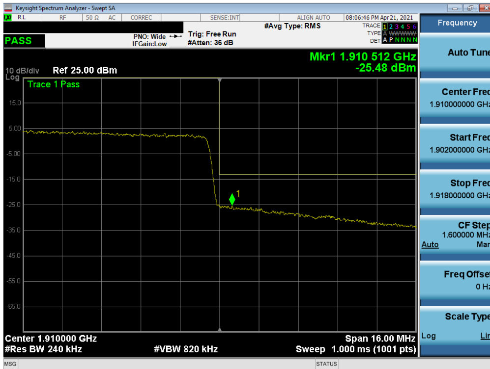
Plot 7-163. Upper Band Edge Plot (NR Band n2 - 20MHz QPSK – Full RB)
