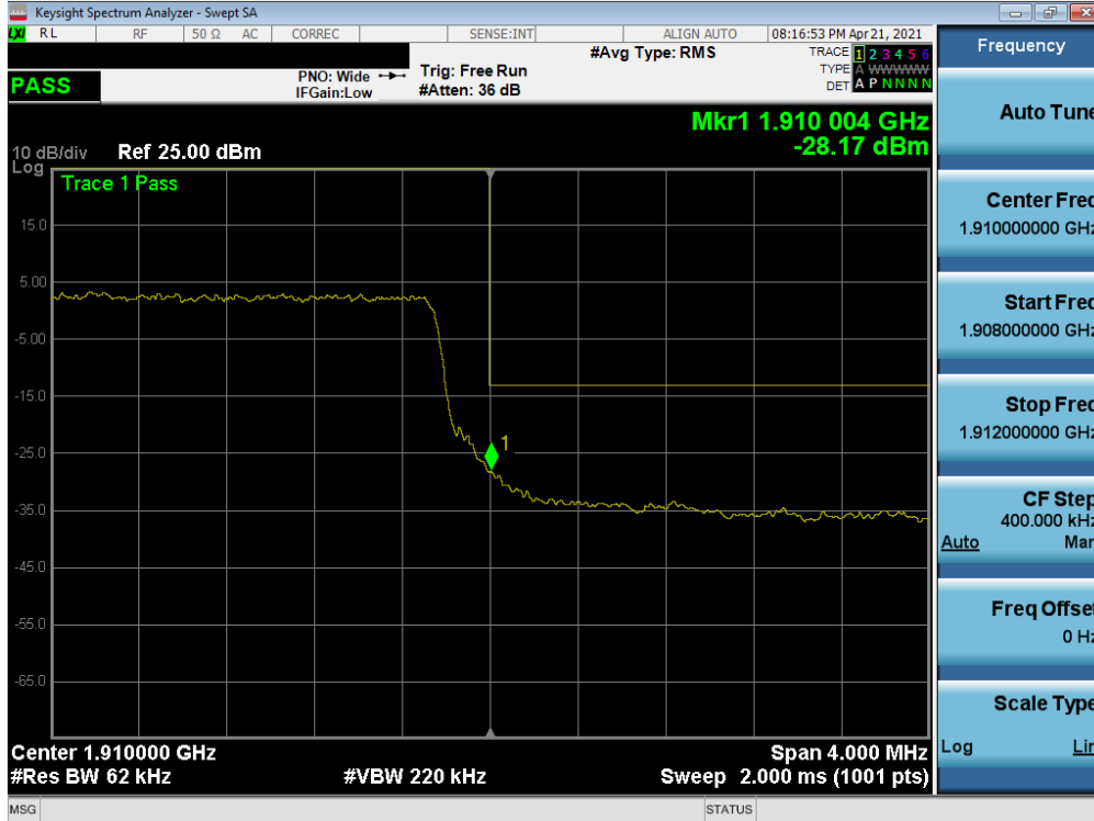
Plot 7-181. Upper Band Edge Plot (NR Band n2 – 5MHz QPSK – Full RB)
