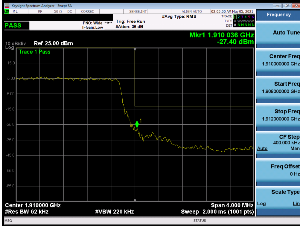
Plot 7-217. Upper Band Edge Plot (NR Band n2 – 5MHz QPSK – Full RB)
