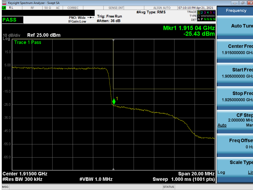
Plot 7-159. Upper Band Edge Plot (NR Band n25 - 25MHz QPSK – Full RB)
