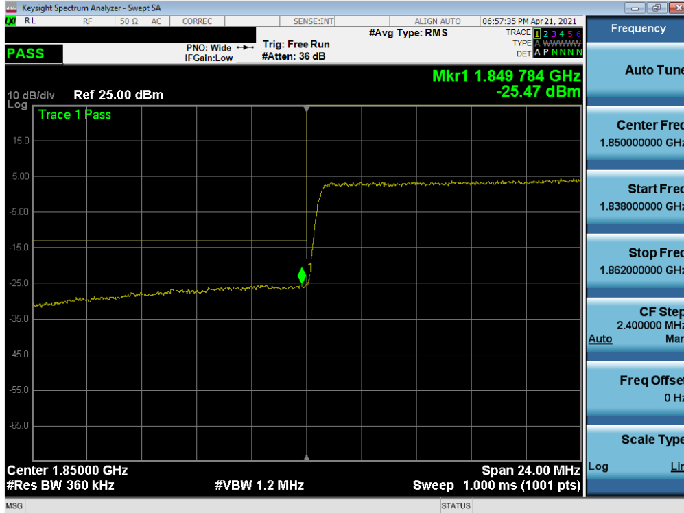
Plot 7-153. Lower Band Edge Plot (NR Band n25 - 30MHz QPSK – Full RB)
