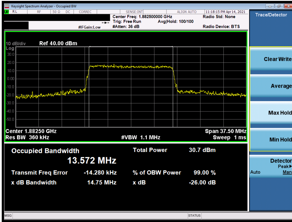
Plot 7-3. Occupied Bandwidth Plot (LTE Band 25/2 - 15MHz QPSK - Full RB)
