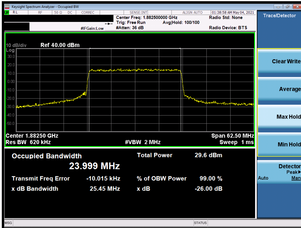
Plot 7-41. Occupied Bandwidth Plot (NR Band n25 - 25.0MHz CP-OFDM QPSK - Full RB)
