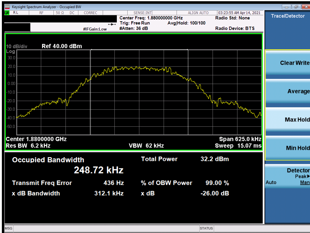
Plot 7-56. Occupied Bandwidth Plot (EDGE, Ch. 661)
