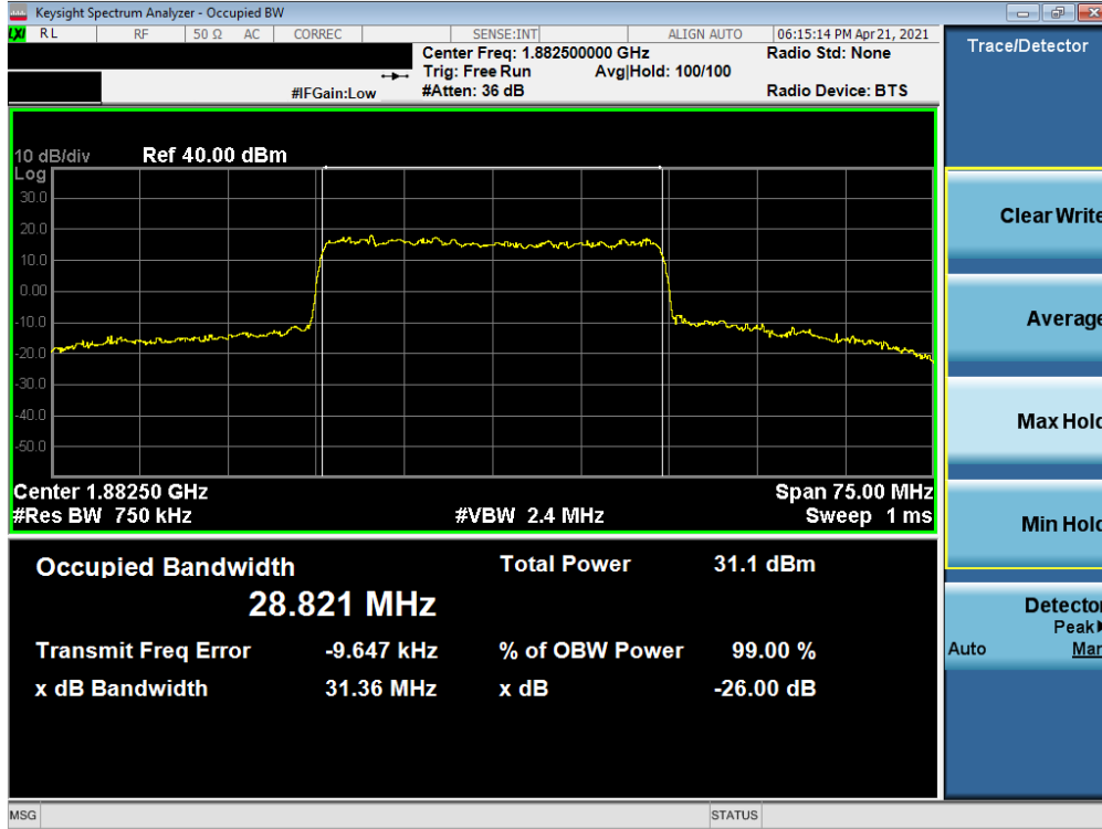
Plot 7-17. Occupied Bandwidth Plot (NR Band n25 - 30.0MHz CP-OFDM QPSK - Full RB)
