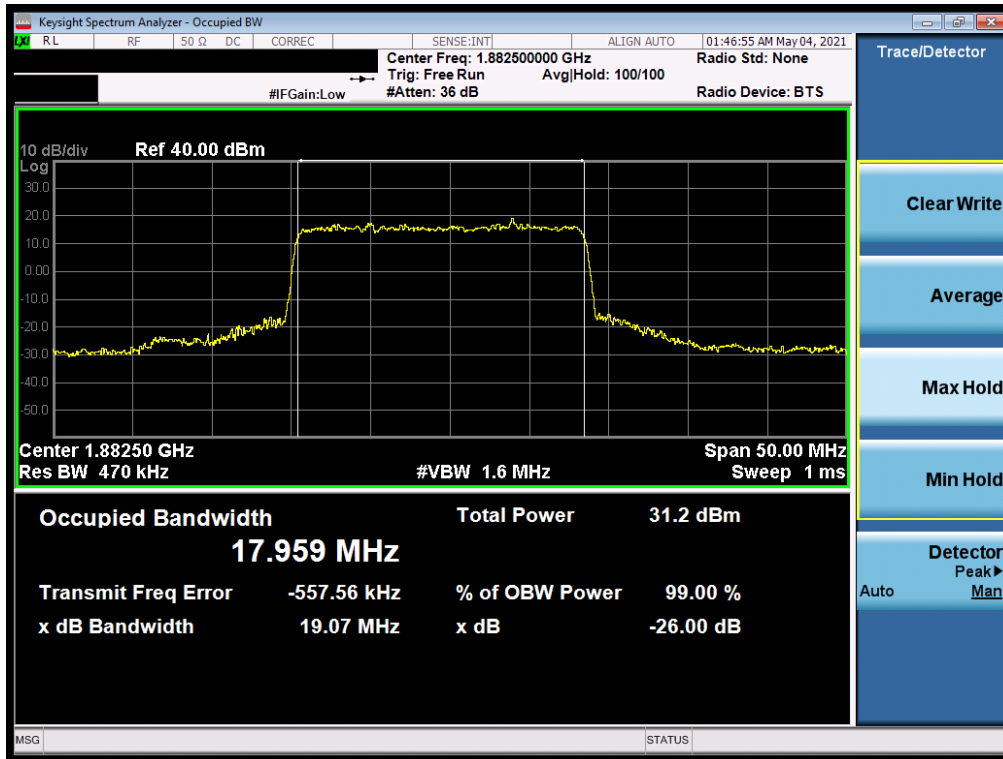
Plot 7-43. Occupied Bandwidth Plot (NR Band n25/2 - 20.0MHz DFT-s-OFDM BPSK - Full RB)
