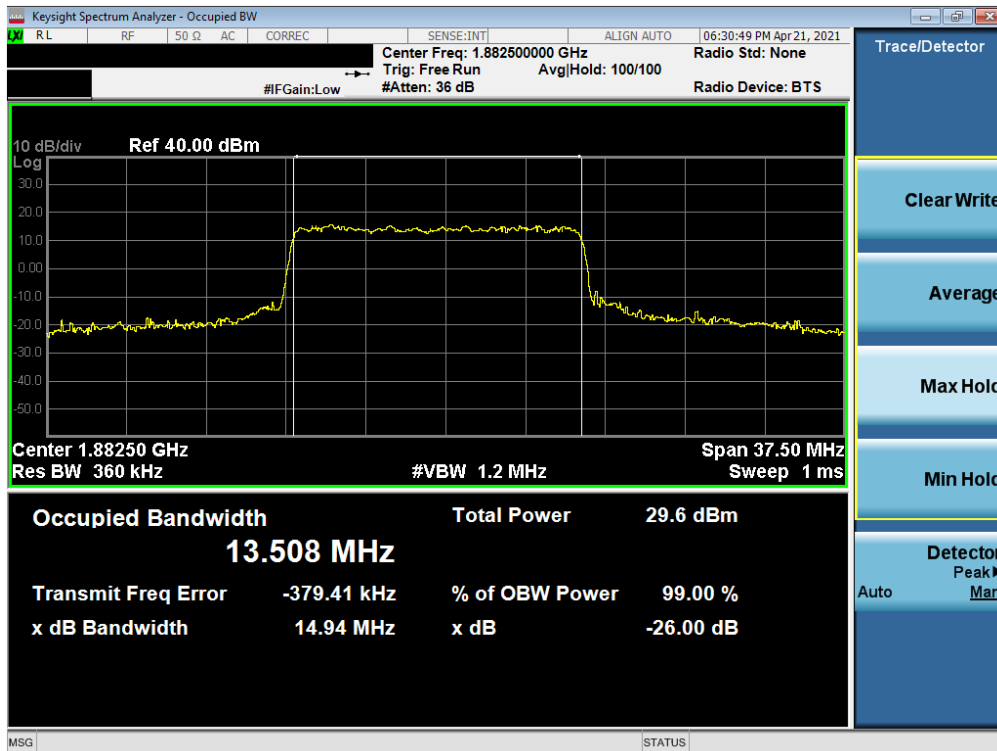
Plot 7-27. Occupied Bandwidth Plot (NR Band n25/2 - 15.0MHz CP-OFDM 16QAM - Full RB)
