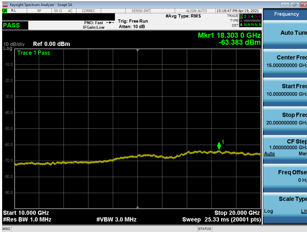
Plot 7-73. Conducted Spurious Plot (NR Band n25/2 - 20.0MHz - 1RB - Mid Channel)
