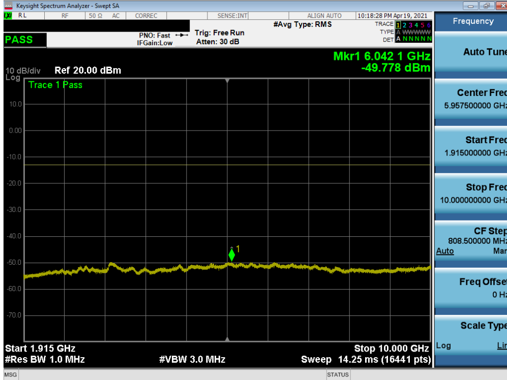
Plot 7-72. Conducted Spurious Plot (NR Band n25/2 - 20.0MHz - 1RB - Mid Channel)
