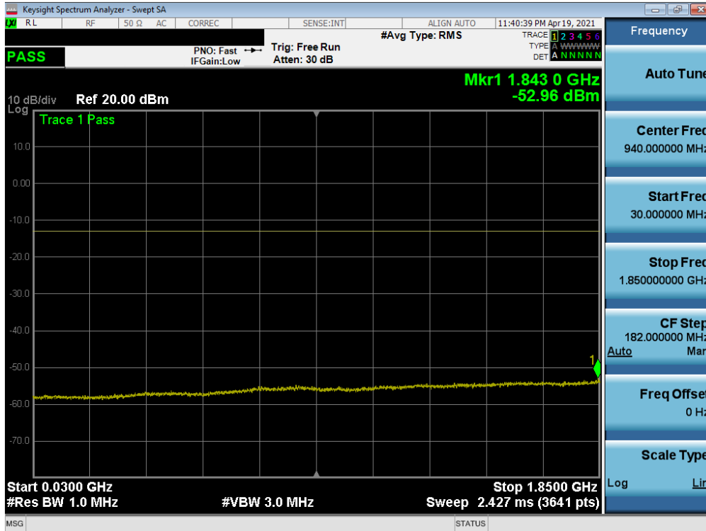
Plot 7-74. Conducted Spurious Plot (NR Band n25/2 - 20.0MHz - 1RB - High Channel)
