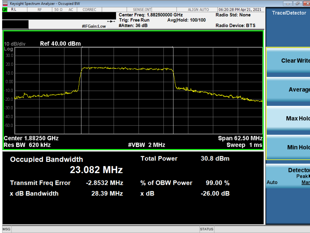
Plot 7-21. Occupied Bandwidth Plot (NR Band n25 - 25.0MHz CP-OFDM 16QAM - Full RB)
