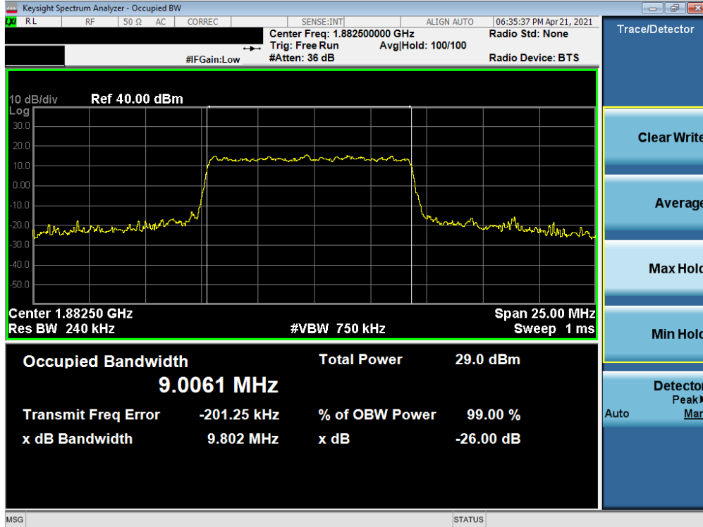
Plot 7-30. Occupied Bandwidth Plot (NR Band n25/2 - 10.0MHz CP-OFDM 16QAM - Full RB)
