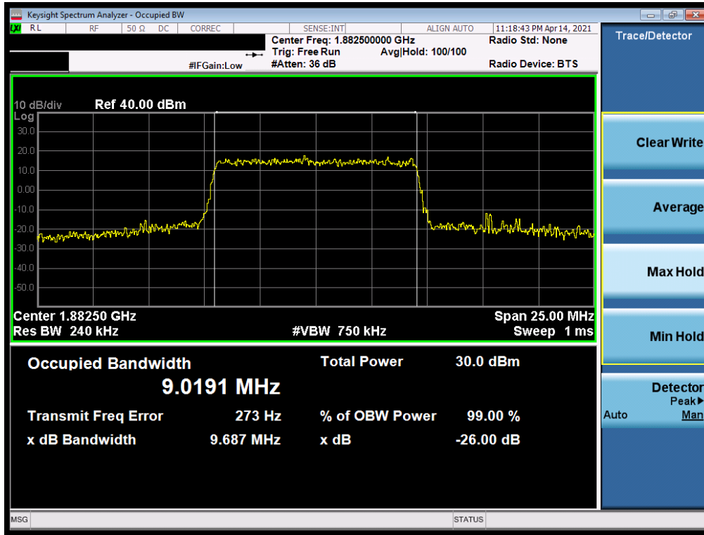
Plot 7-5. Occupied Bandwidth Plot (LTE Band 25/2 - 10MHz QPSK - Full R
