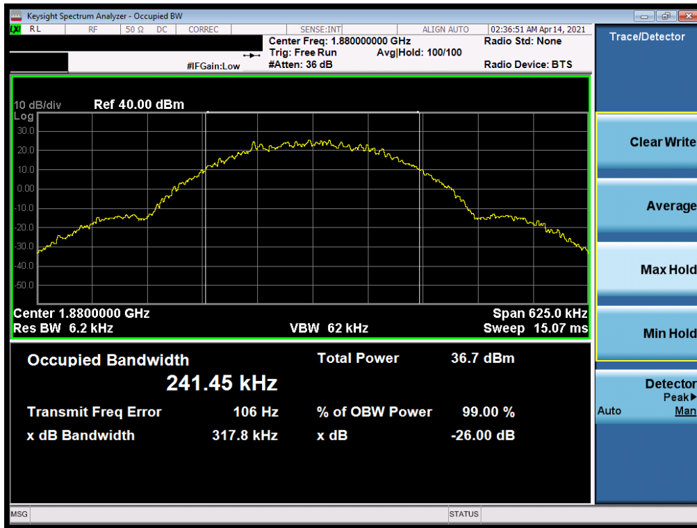
Plot 7-55. Occupied Bandwidth Plot (GPRS, Ch. 661)
