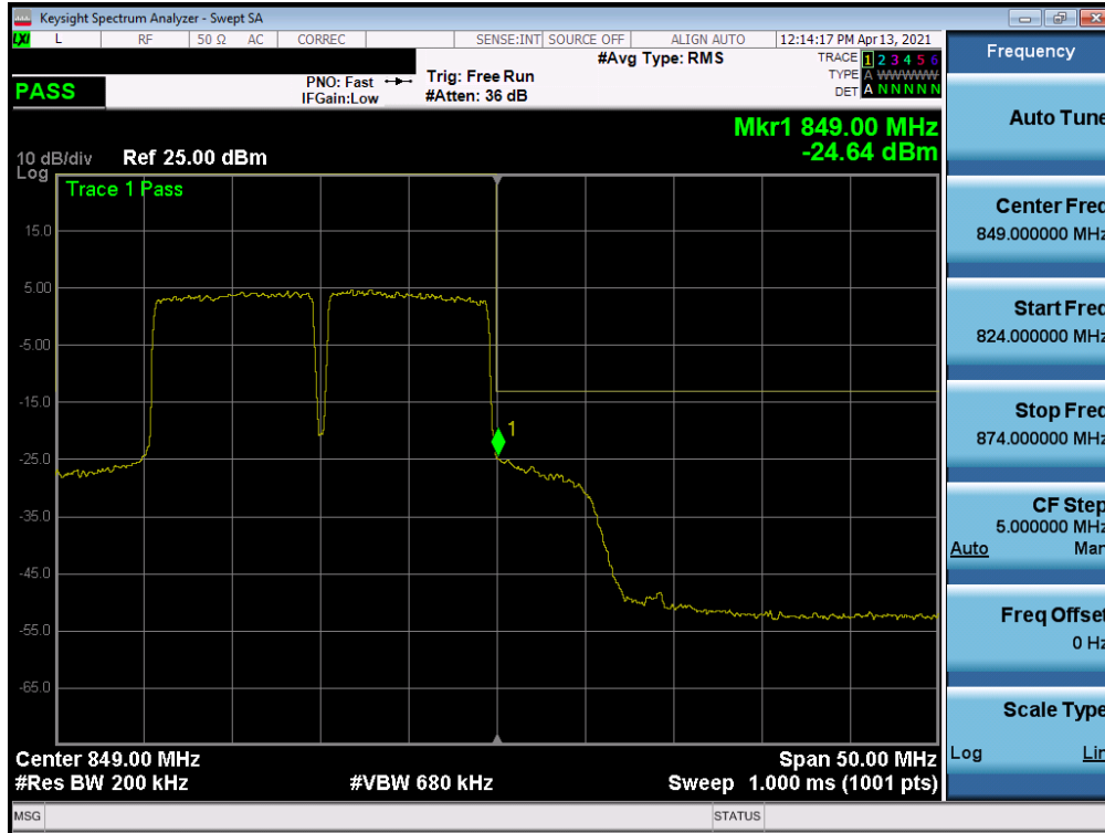
Plot 7-107. Upper Band Edge Plot (Band 5 QPSK – PCC: 10MHz SCC: 10MHz – Full RB)
