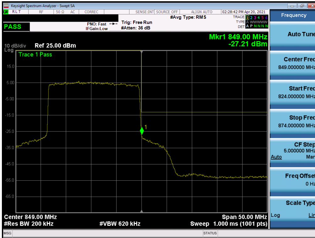
Plot 7-83. Upper Band Edge Plot (NR Band n5 – 20.0MHz QPSK – Full RB)
