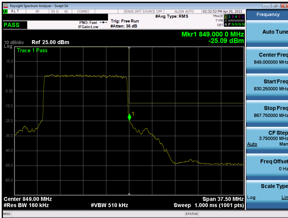
Plot 7-85. Upper Band Edge Plot (NR Band n5 – 15.0MHz QPSK – Full RB)
