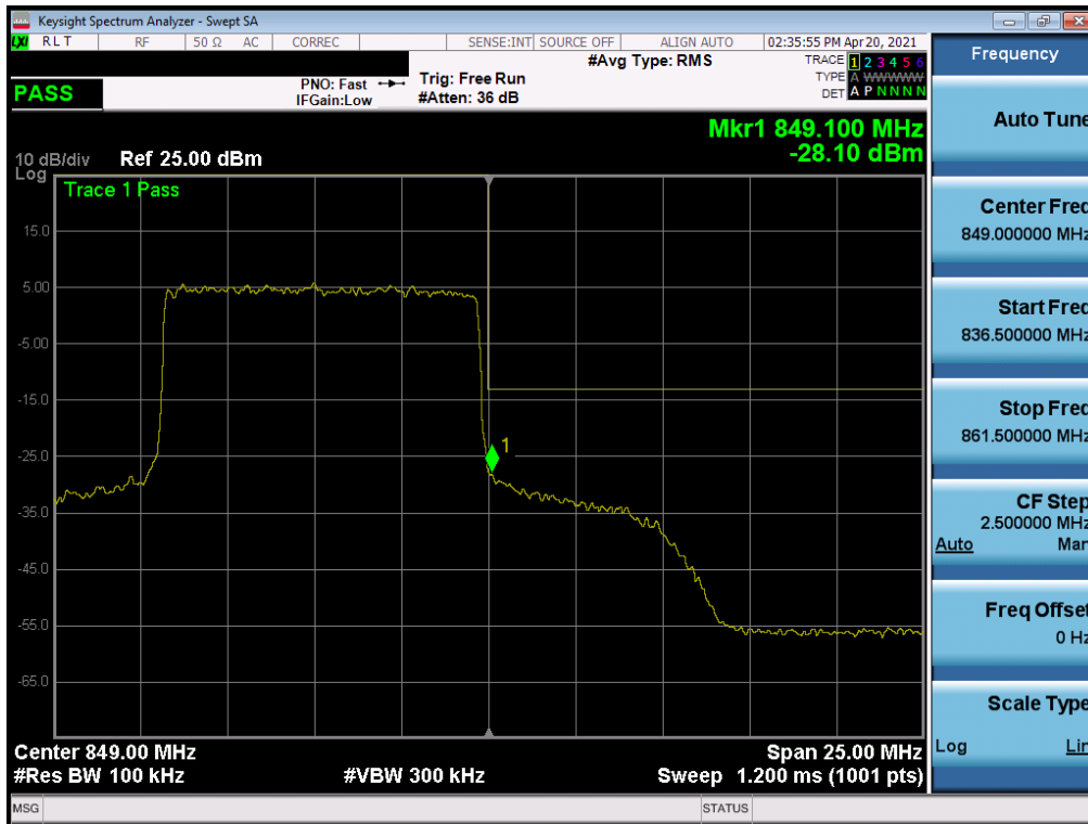
Plot 7-87. Upper Band Edge Plot (NR Band n5 – 10.0MHz QPSK – Full RB)
