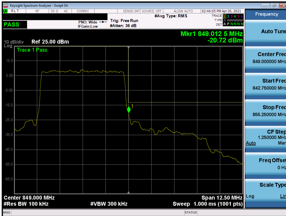
Plot 7-89. Upper Band Edge Plot (NR Band n5 – 5.0MHz QPSK – Full RB)
