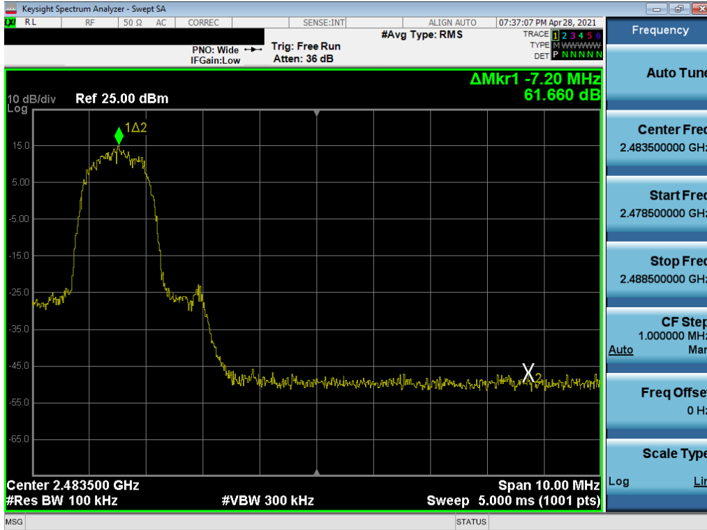
Plot 7-234. Band Edge Plot (Bluetooth with Hopping Disabled, ePA, 3 Mbps – Ch. 78) – ANT1 (N)
