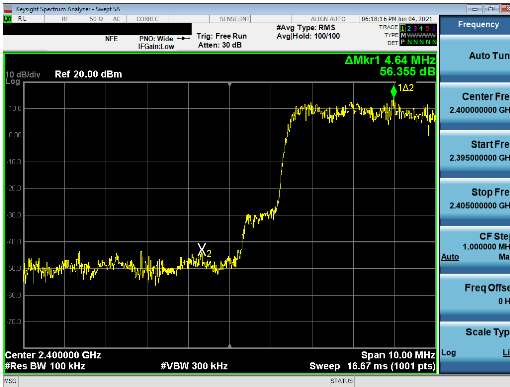
Plot 7-239. Band Edge Plot (Bluetooth with Hopping Enabled, iPA, 3 Mbps – Ch.0) – ANT1 (N)
