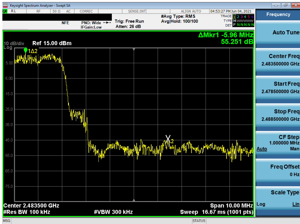
Plot 7-224. Band Edge Plot (Bluetooth with Hopping Enabled, iPA, 3 Mbps – Ch.78) – ANT0 (N)
