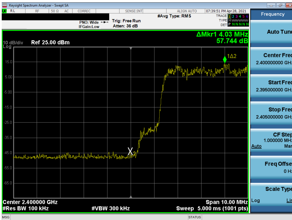
Plot 7-235. Band Edge Plot (Bluetooth with Hopping Enabled, ePA, 3 Mbps – Ch.0) – ANT1 (N)
