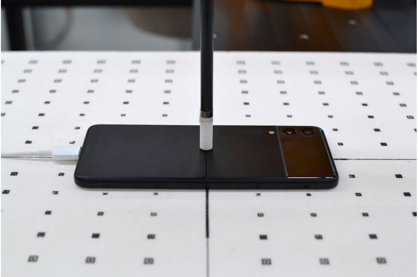
Figure D-6 Near Field Power Density Test Setup Photo – Back Side Open at 2mm
