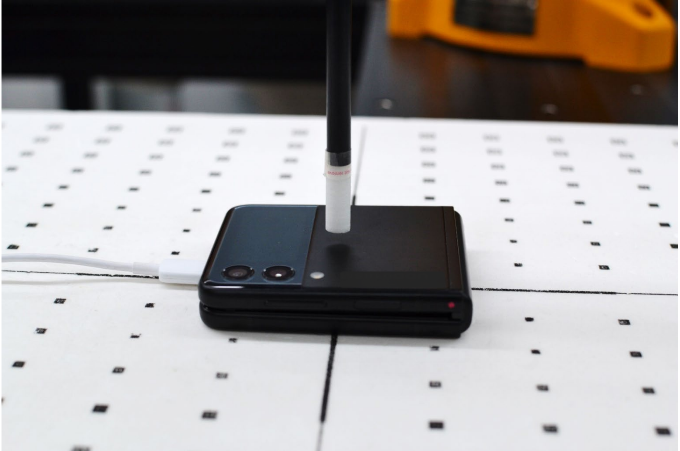
Figure D-9 Near Field Power Density Test Setup Photo – Front Side Closed at 5mm
