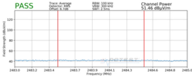
Plot 7-175. Radiated Restricted Upper Band Edge Measurement MIMO (Average – 242 Tones) - N
