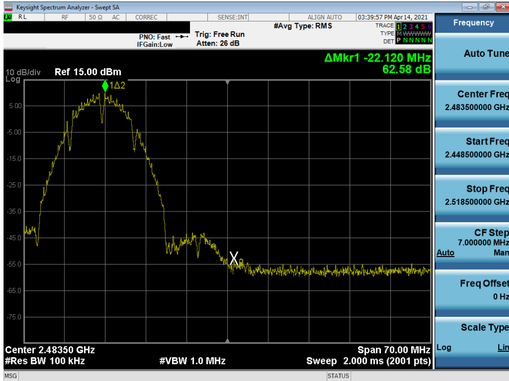
Plot 7-106. Band Edge Plot SISO ANT2 (802.11b – Ch. 11) – N
