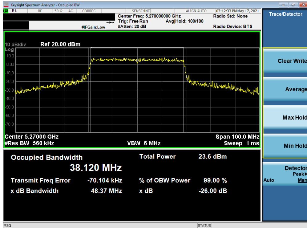
Plot 7-115. 26dB Bandwidth Plot SISO ANT1 (40MHz BW 802.11ax – 484 Tones (UNII Band 2A) – Ch. 54)
