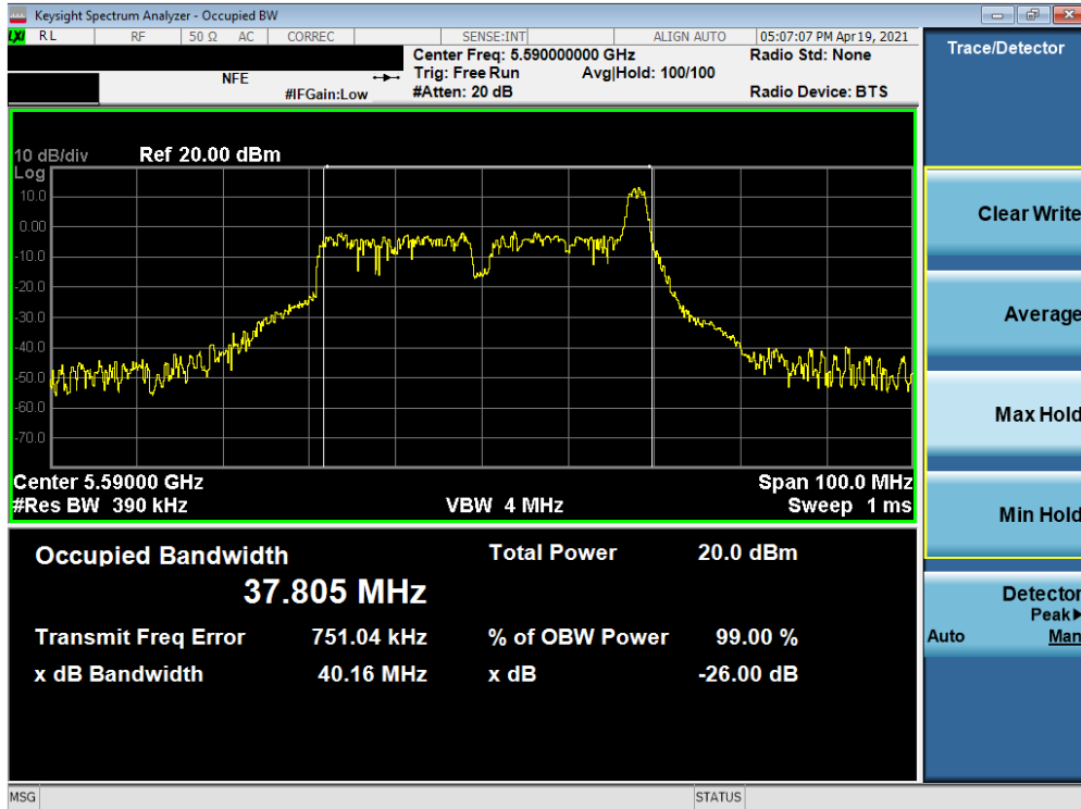
Plot 7-17. 26dB Bandwidth Plot SISO ANT1 (40MHz BW 802.11ax – 26 Tones (UNII Band 2C) – Ch. 118)
