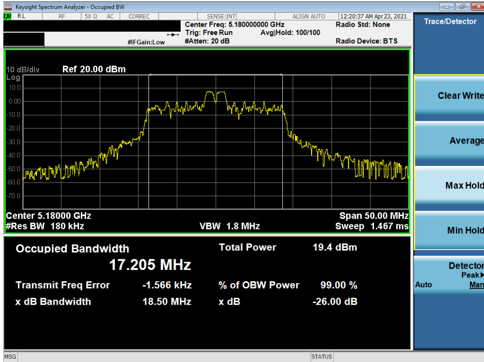
Plot 7-85. 26dB Bandwidth Plot SISO ANT1 (20MHz BW 802.11ax – 26 Tones (UNII Band 1) – Ch. 36)
