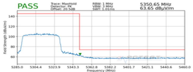
Plot 7-814. Radiated Upper Band Edge Plot MIMO (Peak – UNII Band 2A)
