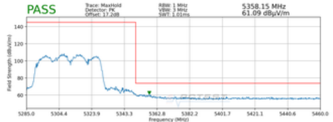
Plot 7-787. Radiated Upper Band Edge Plot MIMO (Peak – UNII Band 2A)
