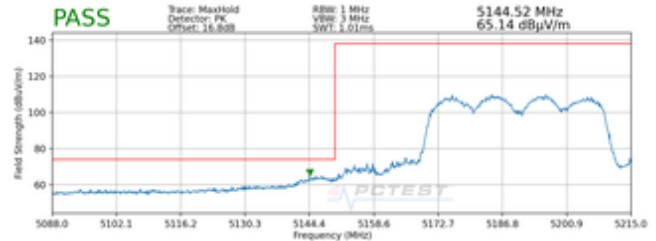
Plot 7-785. Radiated Lower Band Edge Plot MIMO (Peak – UNII Band 1)
