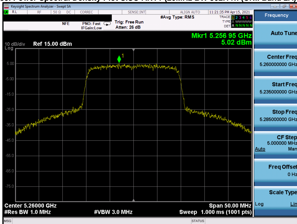
Plot 7-286. Power Spectral Density Plot SISO ANT1 (20MHz BW 802.11ax (UNII Band 2A) – Ch. 52)
