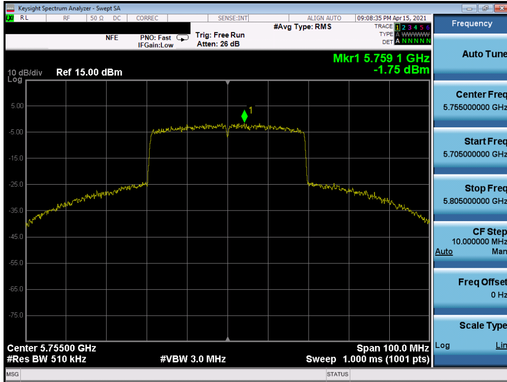
Plot 7-327. Power Spectral Density Plot SISO ANT1 (40MHz BW 802.11ax (UNII Band 3) – Ch. 151)
