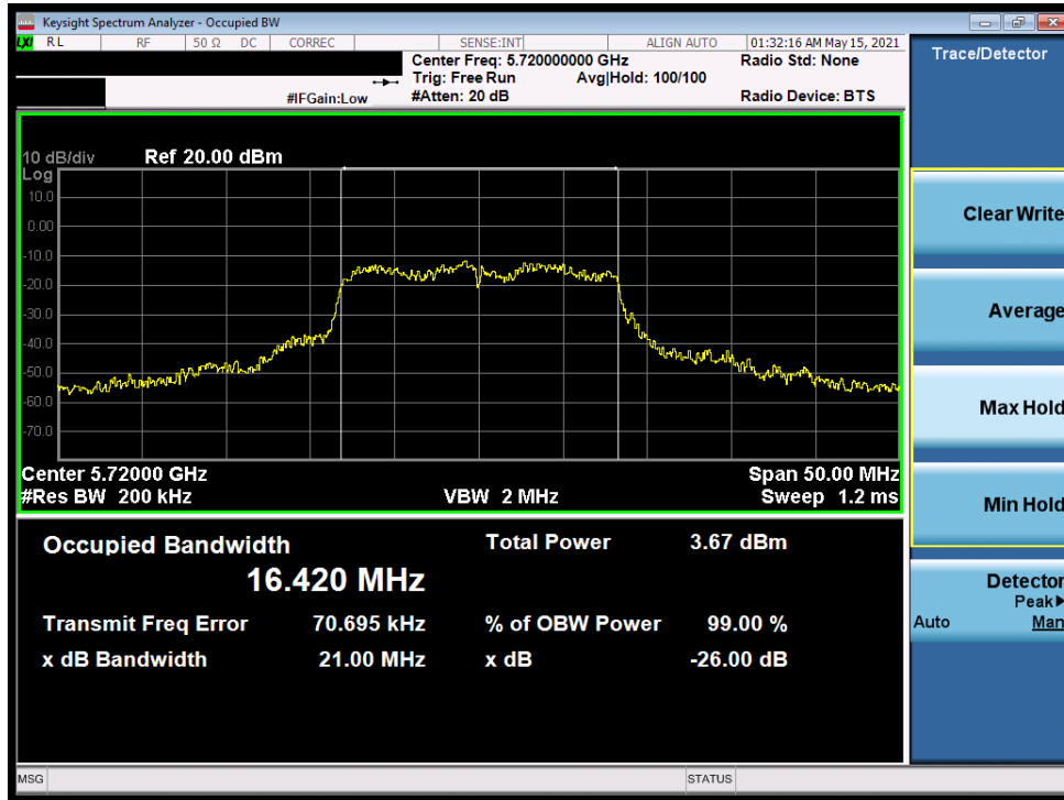
Plot 7-186. 26dB Bandwidth Plot MIMO (20MHz BW 802.11a (UNII Band 2C) – Ch. 144)
