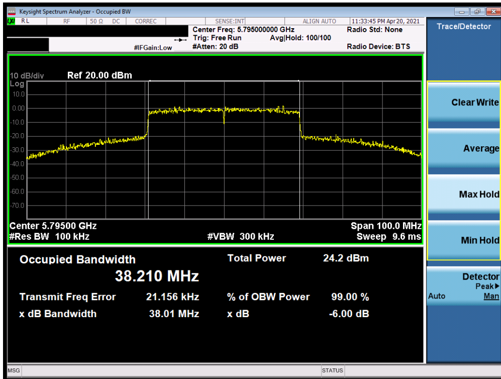
Plot 7-232. 6dB Bandwidth Plot SISO ANT1 (40MHz BW 802.11ax (UNII Band 3) – Ch. 159)
