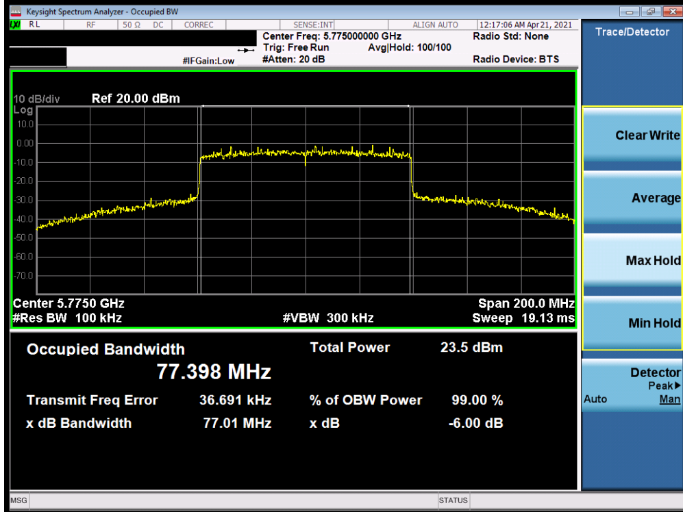
Plot 7-234. 6dB Bandwidth Plot SISO ANT1 (80MHz BW 802.11ax (UNII Band 3) – Ch. 155)
