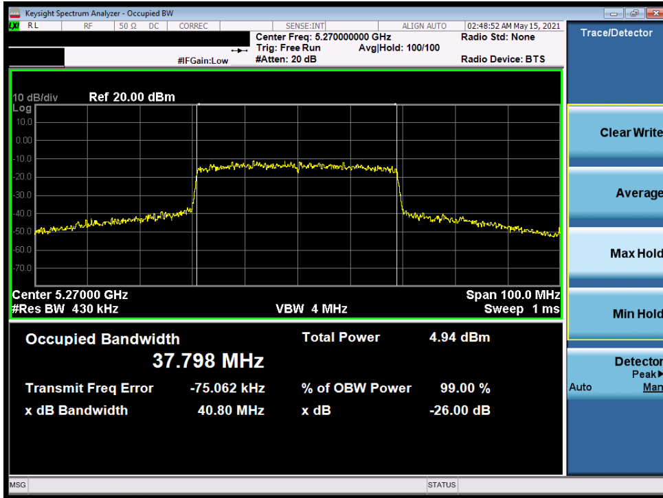
Plot 7-180. 26dB Bandwidth Plot MIMO (40MHz BW 802.11ax (UNII Band 2A) – Ch. 54)
