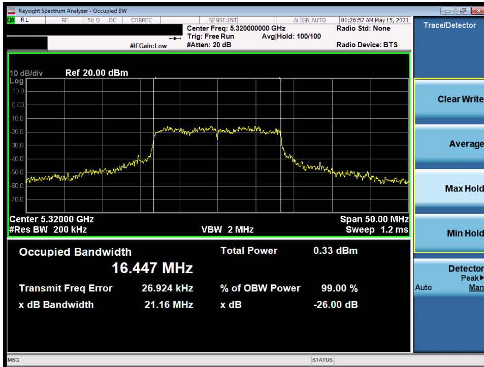
Plot 7-171. 26dB Bandwidth Plot MIMO (20MHz BW 802.11a (UNII Band 2A) – Ch. 64)
