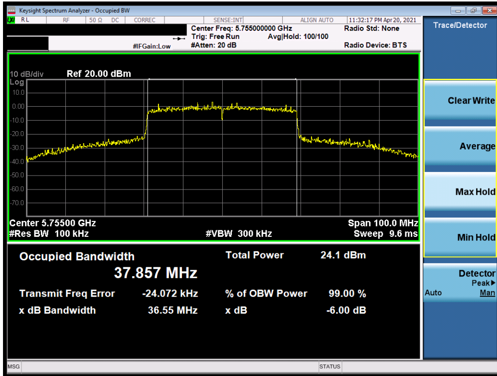
Plot 7-231. 6dB Bandwidth Plot SISO ANT1 (40MHz BW 802.11ax (UNII Band 3) – Ch. 151)
