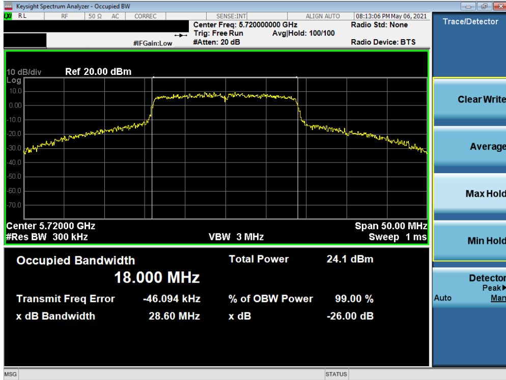
Plot 7-36. 26dB Bandwidth Plot ANT1 (20MHz BW 802.11n (UNII Band 2C) – Ch. 144)
