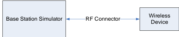
Figure 9-3 Power Measurement Setup
