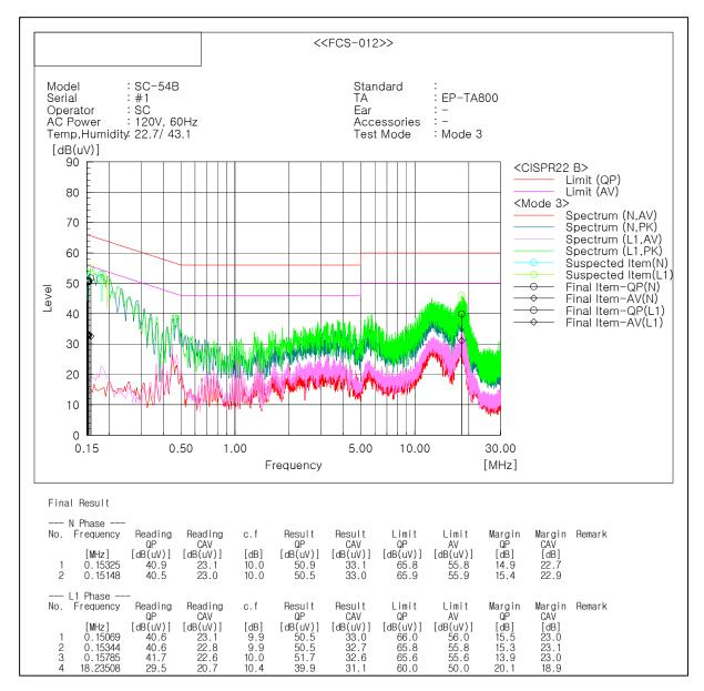
Note 1) Two graphs measured for both Live(L1) and Neutral(N) of the LISN are combined into one graph Note 2) Level (QP and/or CAV) = Meter Reading (QP and/or CAV) + Corr. (LISN Insertion Loss + Cable Loss) Margin (QP and/or CAV) = Limit – Level (QP and/or CAV)
