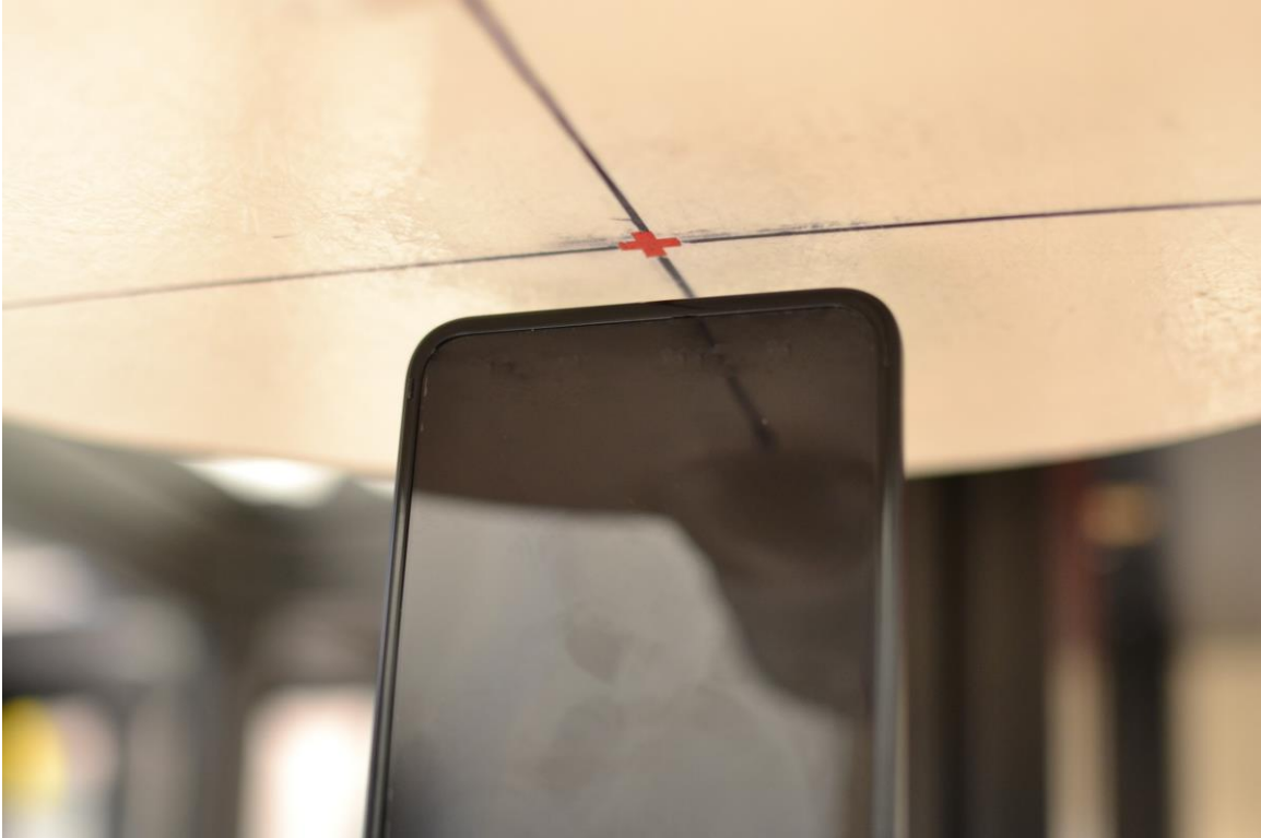
SAR Test Setup Photo 15 – Hotspot, Bottom Edge, 10 mm
