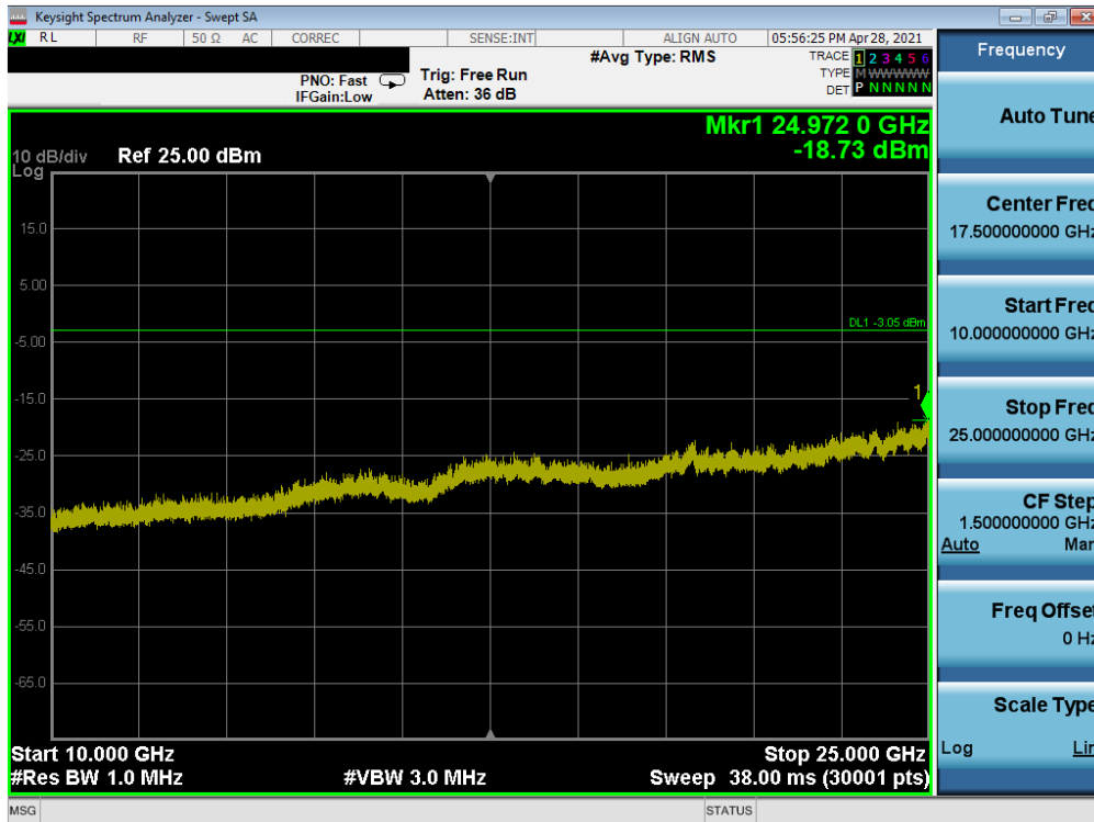
Plot 7-164. Conducted Spurious Plot (Bluetooth, 1Mbps – Ch. 39, ePA) – ANT1
