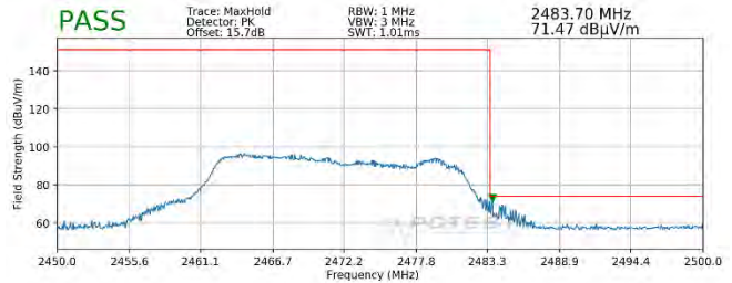
Plot 7-108. Radiated Restricted Upper Band Edge Measurement MIMO (Peak – 242 Tones)
