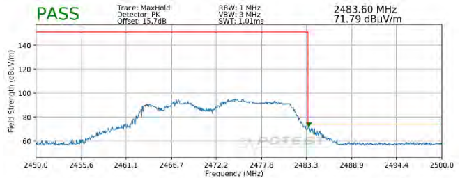
Plot 7-100. Radiated Restricted Upper Band Edge Measurement MIMO (Peak – 106 Tones)
