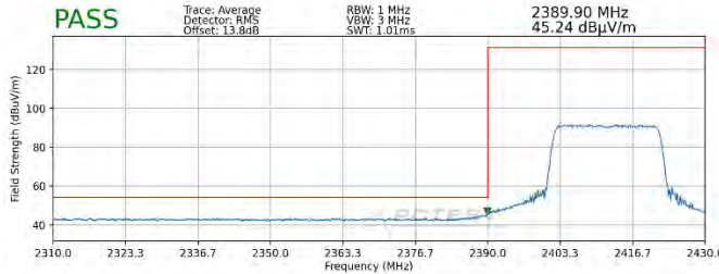
Plot 7-85. Radiated Restricted Lower Band Edge Measurement SISO ANT2 (Average – 242 Tones)
