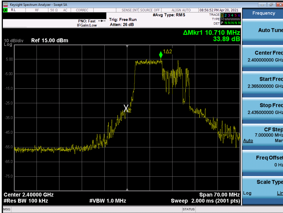
Plot 7-25. Band Edge Plot SISO ANT2 (802.11ax OFDMA – 106 Tones – Ch. 1)
