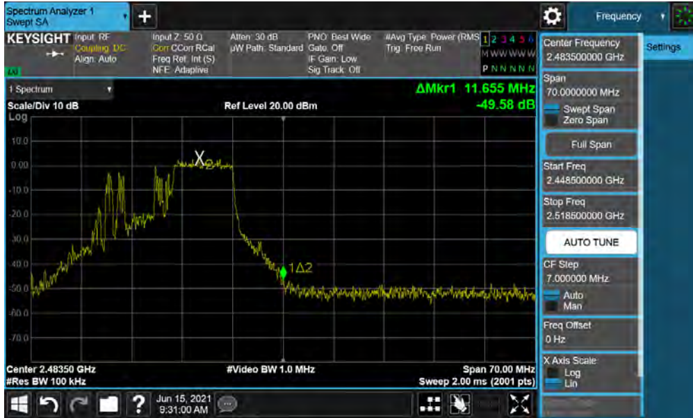
Plot 7-27. Band Edge Plot SISO ANT2 (802.11ax OFDMA – 106 Tones – Ch. 12)
