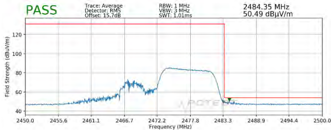
Plot 7-99. Radiated Restricted Upper Band Edge Measurement MIMO (Average – 106 Tones)
