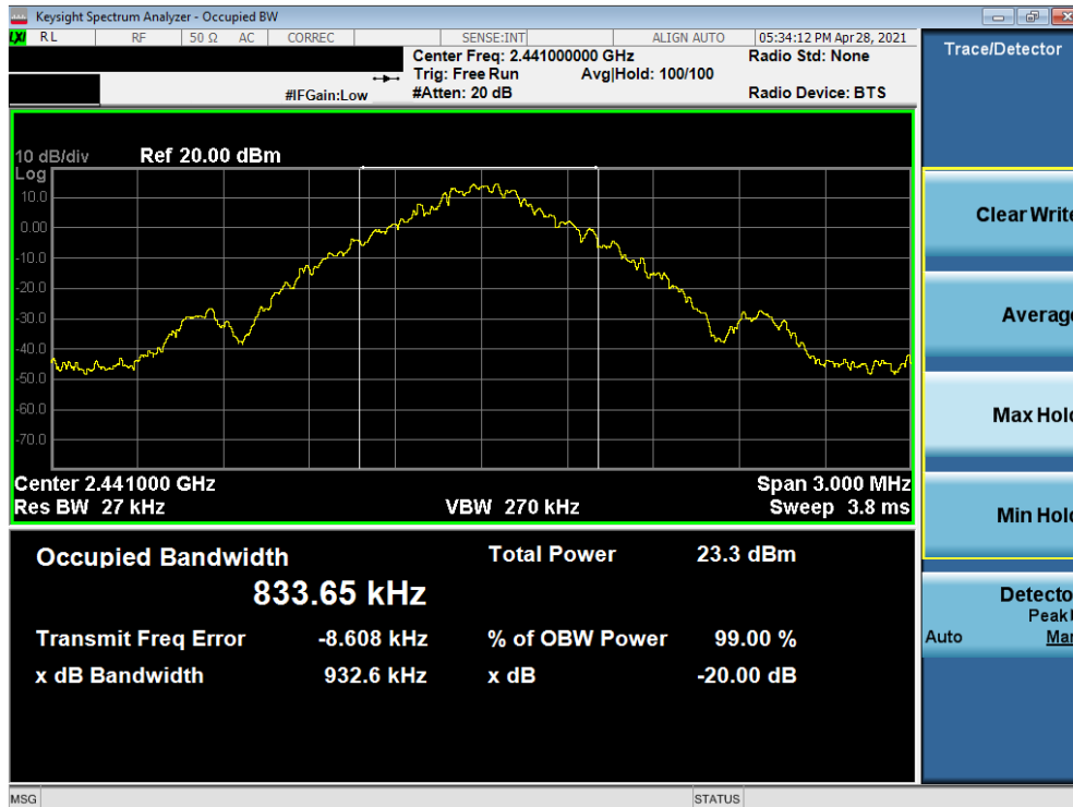
Plot 7-20. 20dB Bandwidth Plot (Bluetooth, 1Mbps, ePA – Ch. 39) – ANT1
