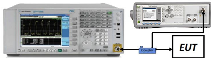
Figure 7-3. Test Instrument & Measurement Setup
