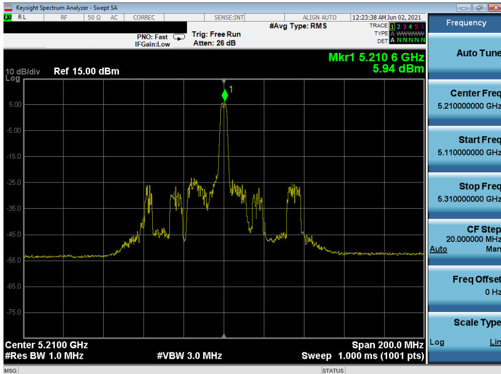
Plot 7-168. Power Spectral Density Plot MIMO ANT1 (80MHz BW 802.11ax – 26 Tones (UNII Band 1) – Ch. 42)
