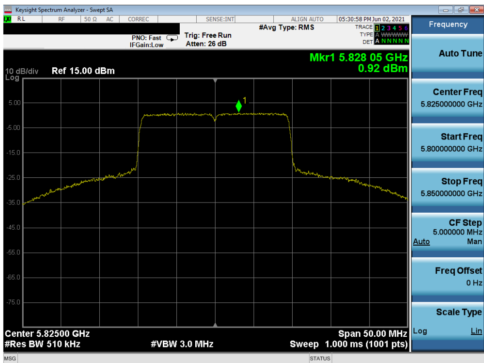
Plot 7-240. Power Spectral Density Plot MIMO ANT1 (20 MHz BW 802.11ax – Full Tones (UNII Band 3) – Ch. 165)
