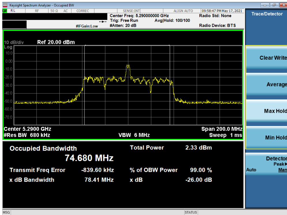
Plot 7-54. 26dB Bandwidth Plot MIMO (80MHz BW 802.11ax – 26 Tones (UNII Band 2A) – Ch. 58)
