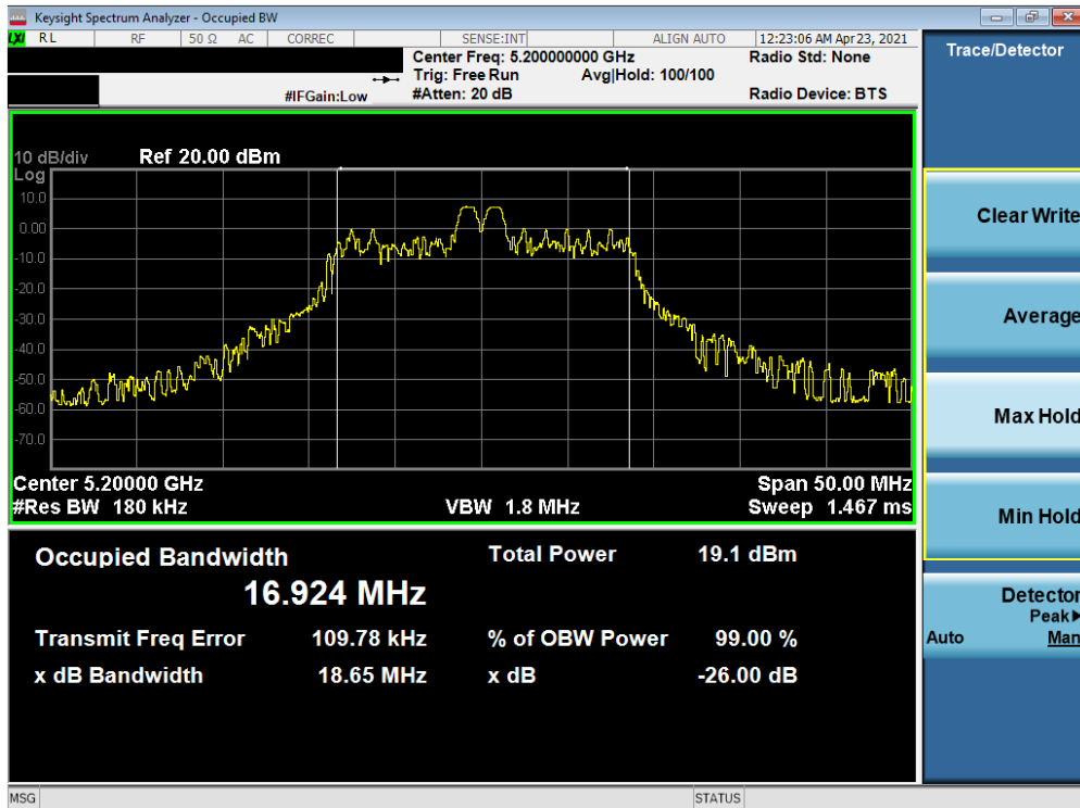
Plot 7-2. 26dB Bandwidth Plot SISO ANT1 (20MHz BW 802.11ax – 26 Tones (UNII Band 1) – Ch. 40)
