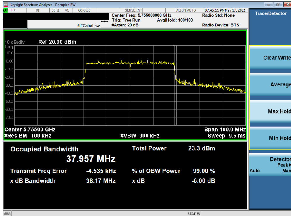
Plot 7-94. 6dB Bandwidth Plot SISO ANT1 (40MHz BW 802.11ax – 484 Tones (UNII Band 3) – Ch. 151)
