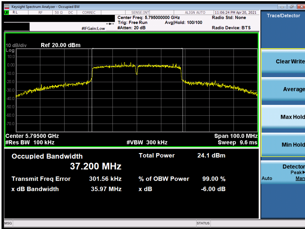
Plot 7-113. 6dB Bandwidth Plot SISO ANT1 (40MHz BW 802.11n (UNII Band 3) – Ch. 159)
