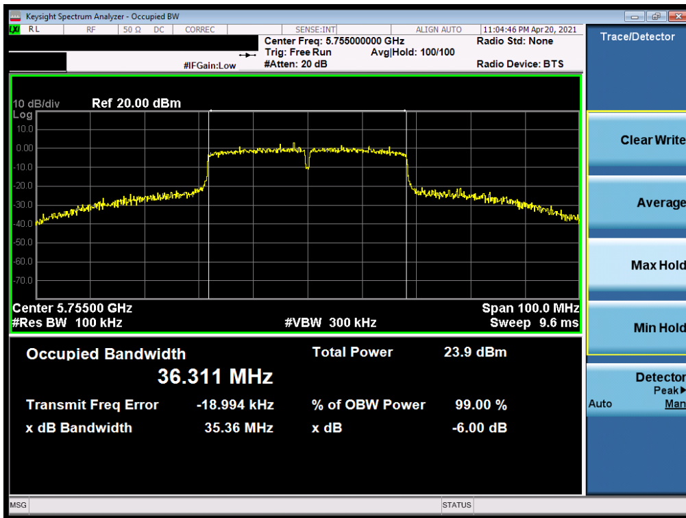
Plot 7-112. 6dB Bandwidth Plot SISO ANT1 (40MHz BW 802.11n (UNII Band 3) – Ch. 151)
