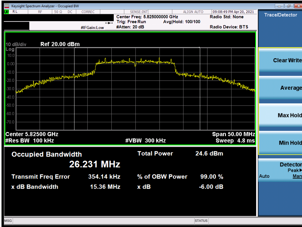
Plot 7-105. 6dB Bandwidth Plot SISO ANT1 (20MHz BW 802.11a (UNII Band 3) – Ch. 165)
