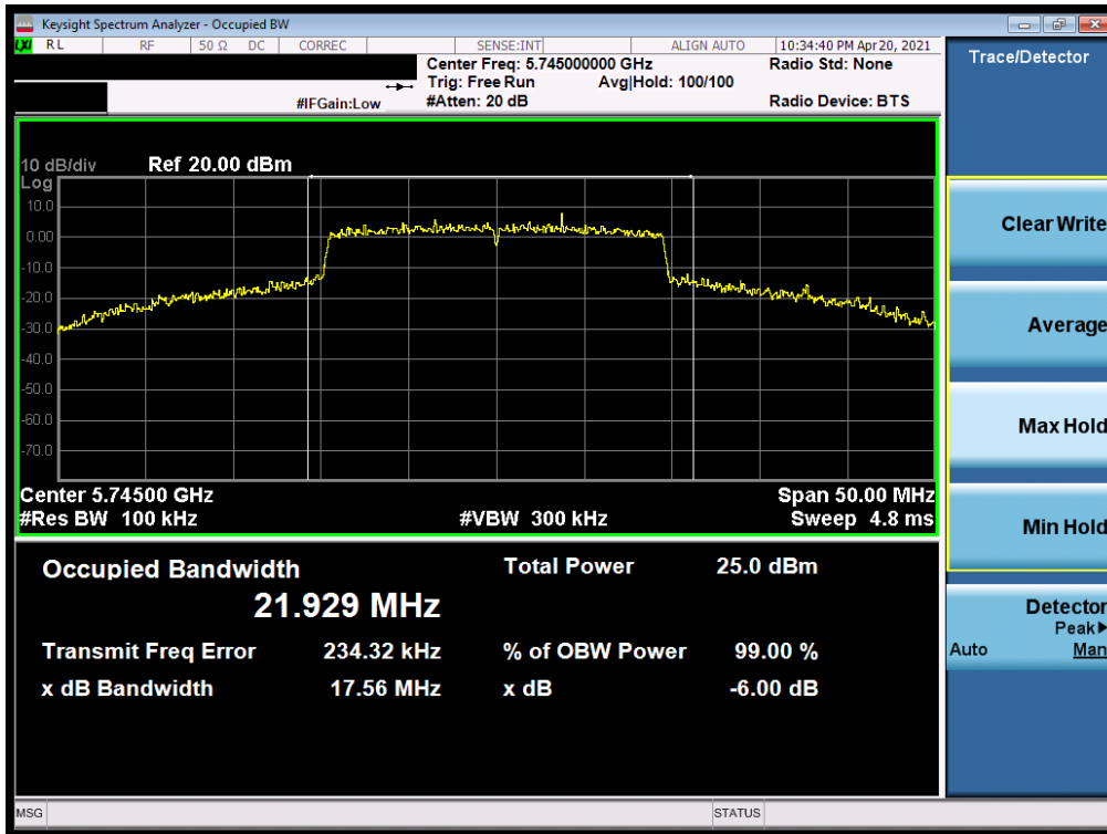
Plot 7-109. 6dB Bandwidth Plot SISO ANT1 (20MHz BW 802.11ax (UNII Band 3) – Ch. 149)
