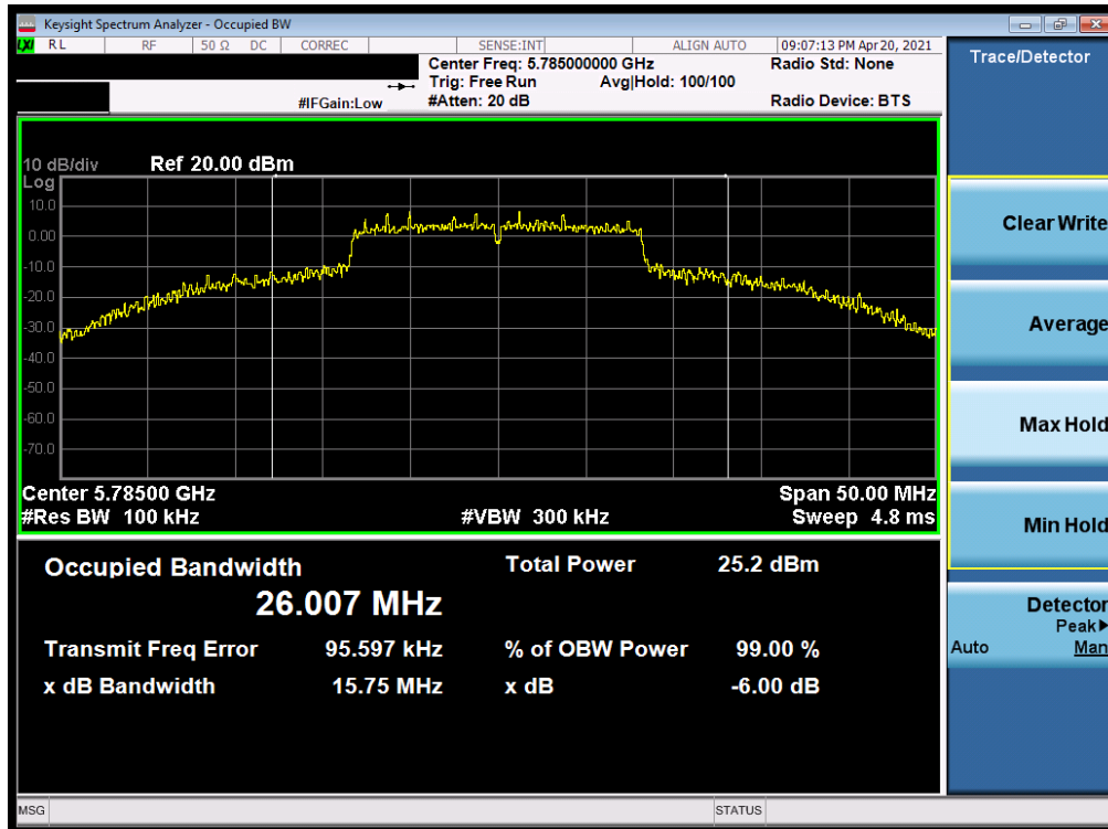
Plot 7-104. 6dB Bandwidth Plot SISO ANT1 (20MHz BW 802.11a (UNII Band 3) – Ch. 157)
