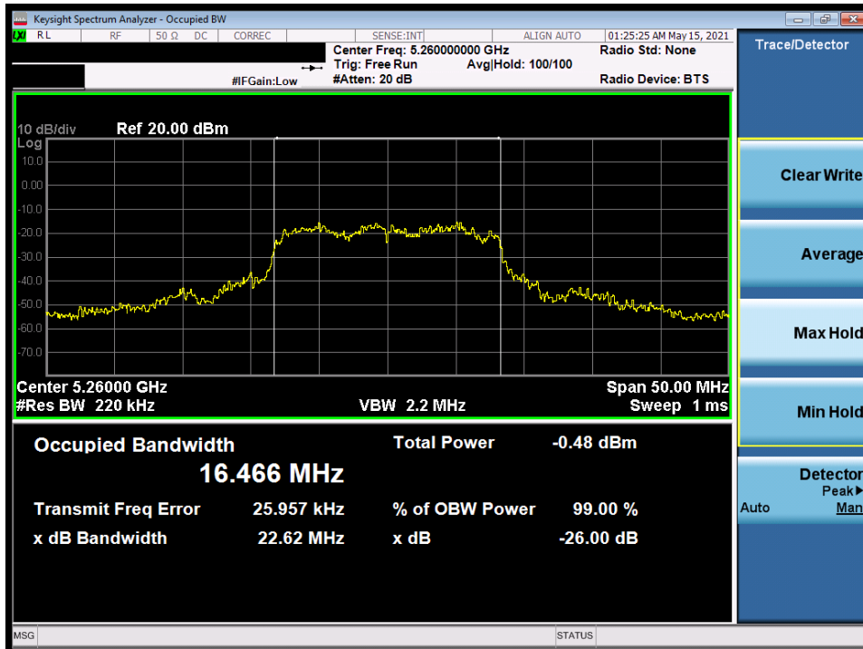
Plot 7-67. 26dB Bandwidth Plot MIMO (20MHz BW 802.11a (UNII Band 2A) – Ch. 52)
