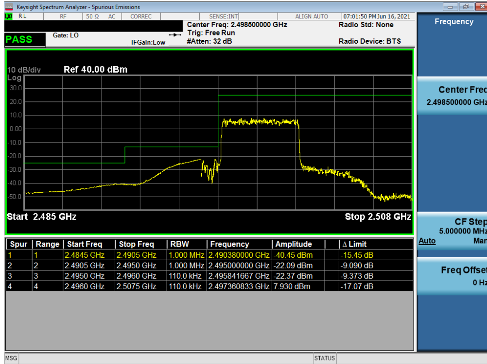
Plot 7-24. Lower ACP Plot (LTE Band 41(PC3) - 5MHz QPSK – Full RB )
