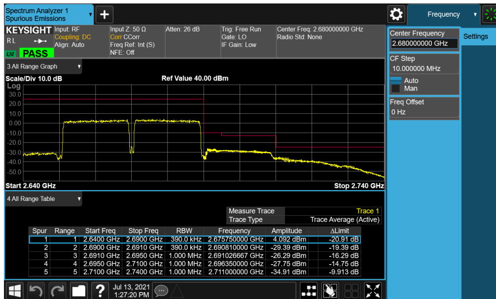
Plot 7-39. Upper ACP Plot (ULCA LTE B41(PC3) - 20MHz QPSK – Full RB)
