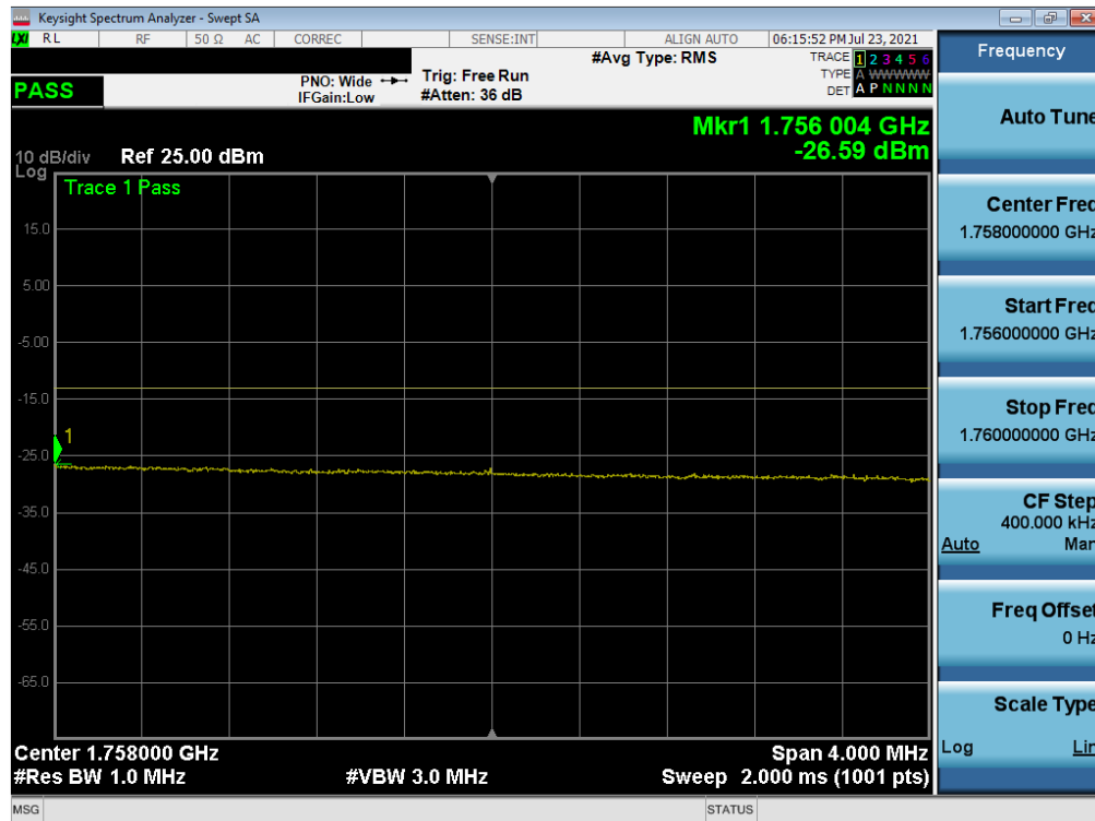
Plot 7-69. Upper Extended Band Edge Plot (LTE Band 4 - 15MHz QPSK – Full RB)
