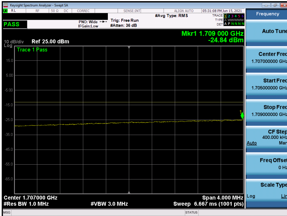
Plot 7-67. Lower Extended Band Edge Plot (LTE Band 4 - 15MHz QPSK – Full RB)
