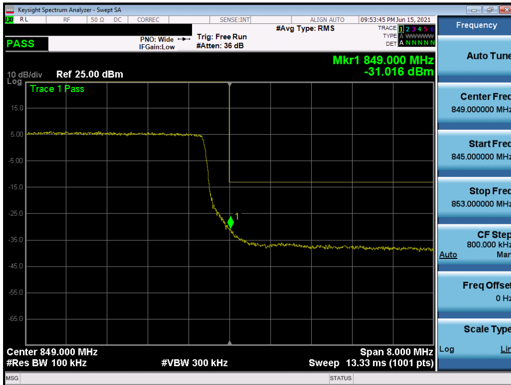
Plot 7-40. Upper Band Edge Plot (LTE Band 5 - 10MHz QPSK – Full RB)
