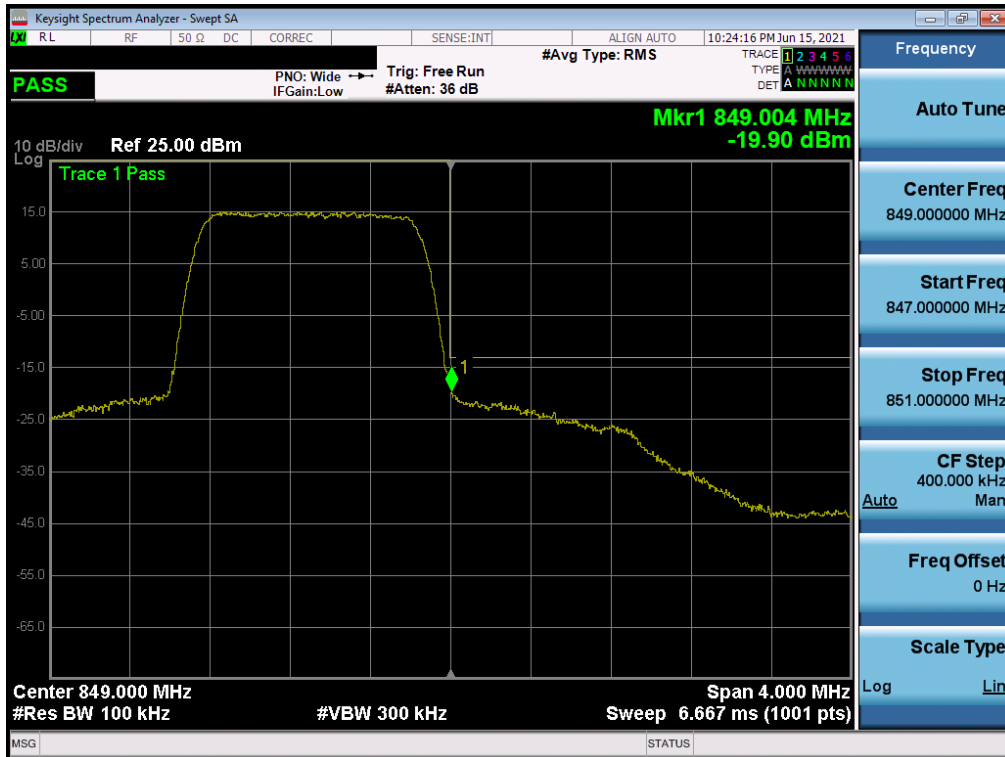
Plot 7-46. Upper Band Edge Plot (LTE Band 5 – 1.4MHz QPSK – Full RB)
