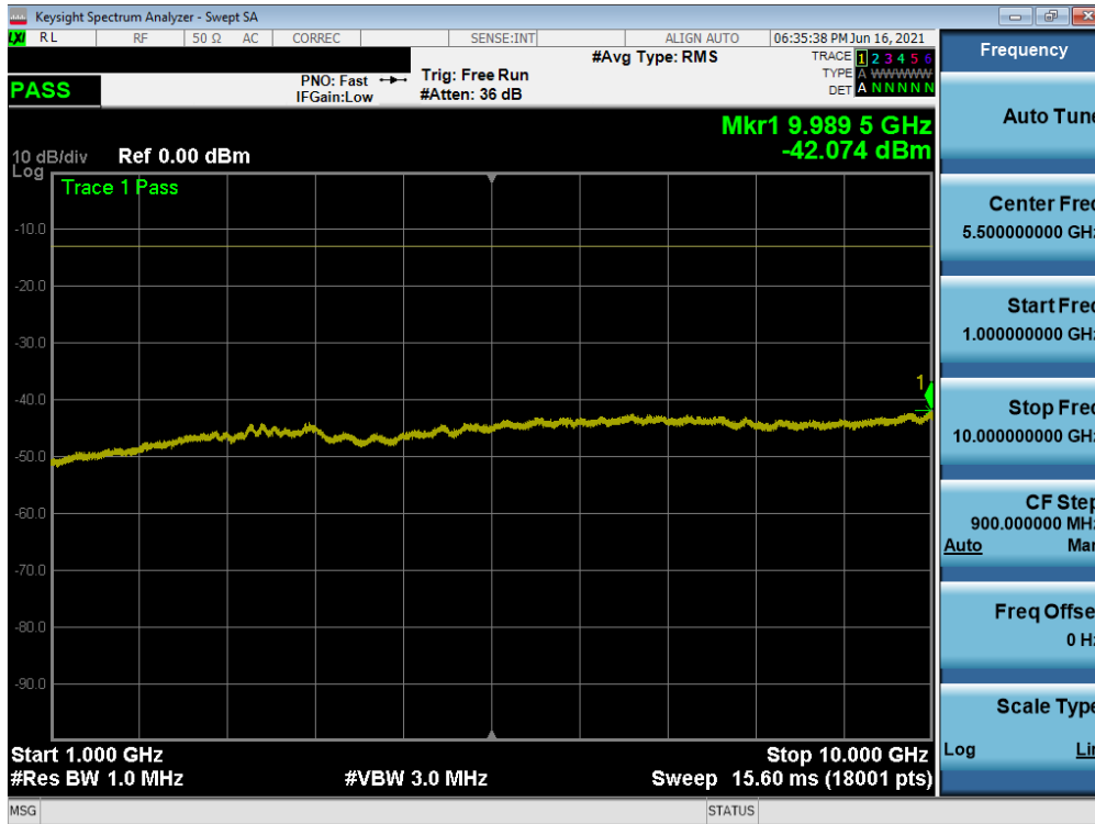
Plot 7-32. Conducted Spurious Plot (WCDMA Ch. 4132)
