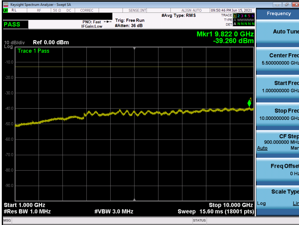
Plot 7-14. Conducted Spurious Plot (LTE Band 5 - 10MHz QPSK - 1 RB - Low Channel)
