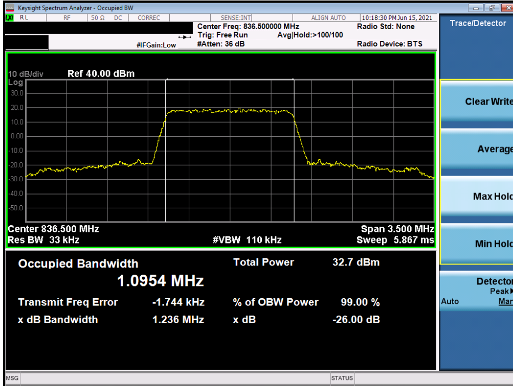
Plot 7-7. Occupied Bandwidth Plot (LTE Band 5 - 1.4MHz QPSK - Full RB)
