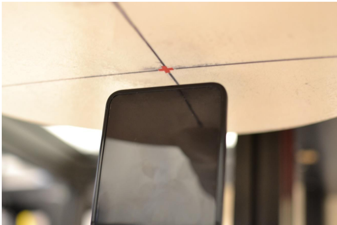
SAR Test Setup Photo 14 – Phablet, Bottom Edge at 11 mm
