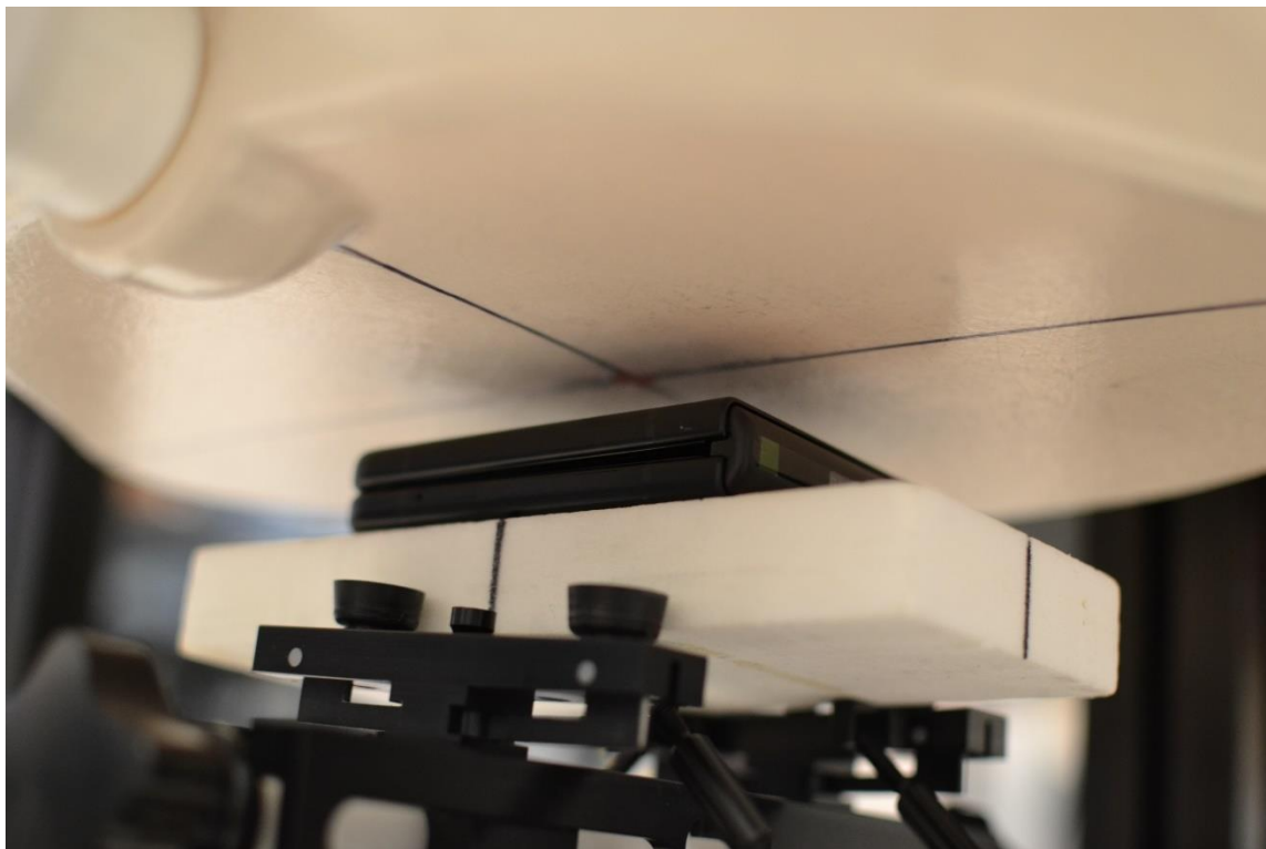
SAR Test Setup Photo 22 – Closed Body-Worn, Back Side, 15 mm
