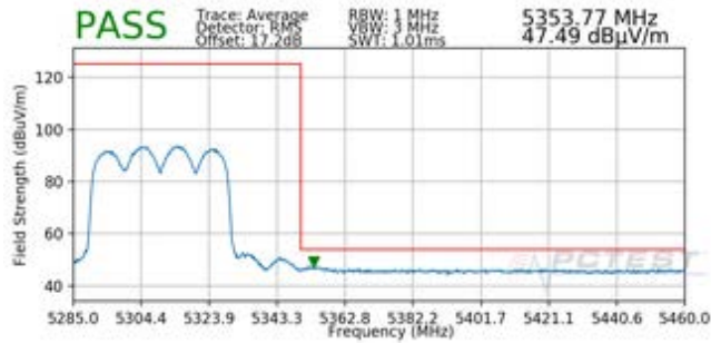
Plot 7-401. Radiated Upper Band Edge Plot MIMO with WCP (Average – UNII Band 2A)
