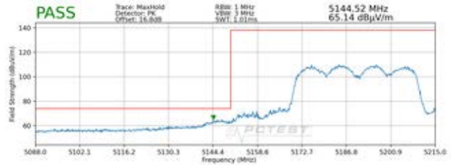
Plot 7-395. Radiated Lower Band Edge Plot MIMO (Peak – UNII Band 1)
