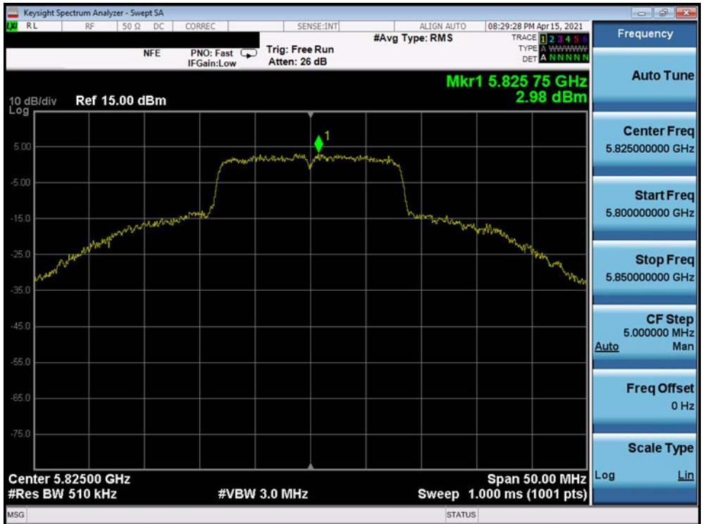
Plot 7-186. Power Spectral Density Plot SISO ANT1 (20MHz 802.11a (UNII Band 3) – Ch. 165)
