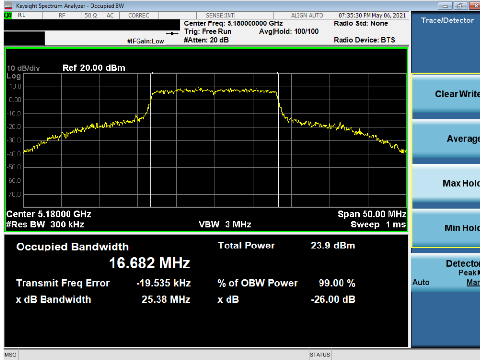
Plot 7-1. 26dB Bandwidth Plot SISO ANT1 (20MHz 802.11a (UNII Band 1) – Ch. 36)
