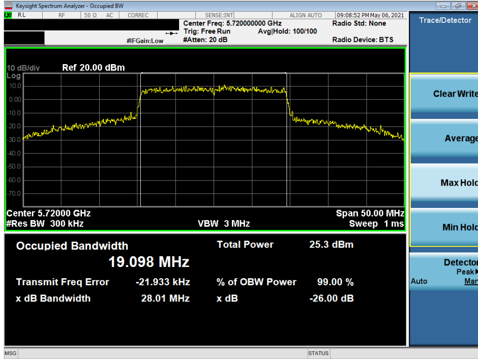
Plot 7-39. 26dB Bandwidth Plot SISO ANT1 (20MHz 802.11ax (UNII Band 2C) – Ch. 144)
