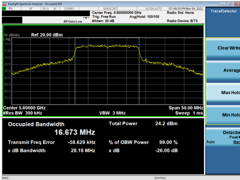
Plot 7-32. 26dB Bandwidth Plot SISO ANT1 (20MHz 802.11a (UNII Band 2C) – Ch. 120)
