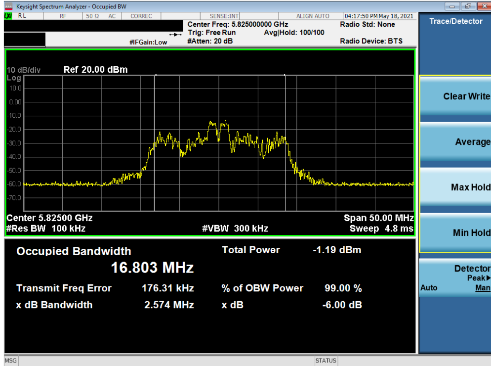
Plot 7-99. 6dB Bandwidth Plot MIMO (20MHz BW 802.11ax – 26 Tones (UNII Band 3) – Ch. 165)
