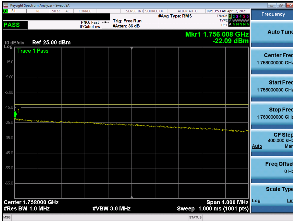
Plot 7-114. Upper Extended Band Edge Plot (LTE Band 4 - 10MHz QPSK – Full RB)
