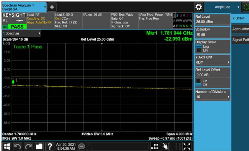
Plot 7-138. Upper Extended Band Edge Plot (NR Band n66 – 20.0MHz - Full RB)
