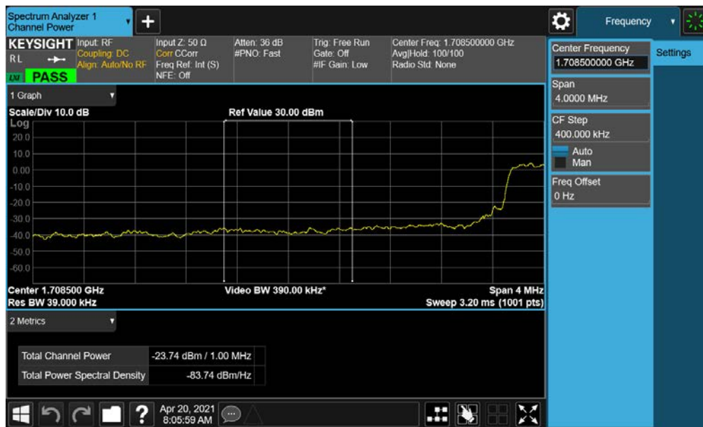
Plot 7-148. Lower Extended Band Edge Plot (NR Band n66 – 5.0MHz - Full RB)
