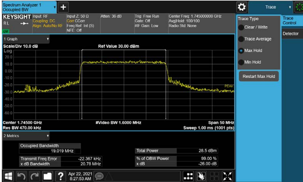
Plot 7-28. Occupied Bandwidth Plot (NR Band n66 - 20.0MHz CP-OFDM 16QAM - Full RB)
