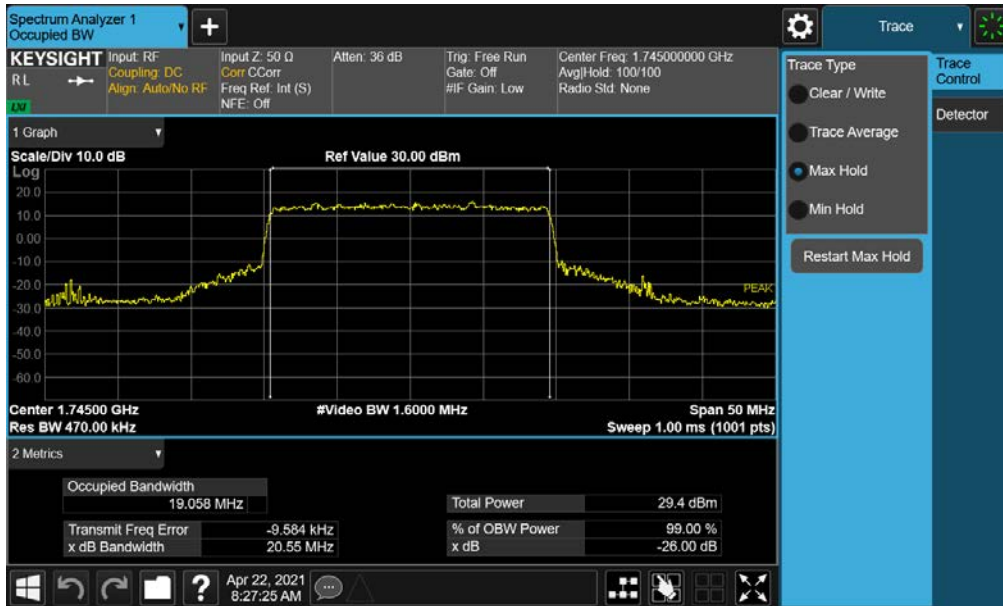
Plot 7-27. Occupied Bandwidth Plot (NR Band n66 - 20.0MHz CP-OFDM QPSK - Full RB)
