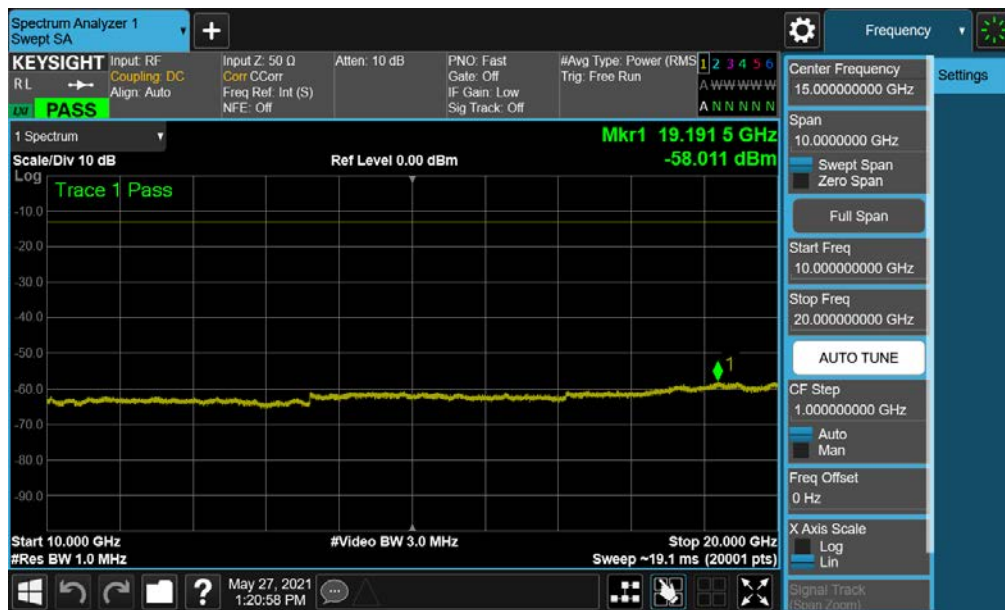
Plot 7-73. Conducted Spurious Plot (NR Band n66 - 20.0MHz - RB Size 1, RB Offset 0 - Mid Channel)
