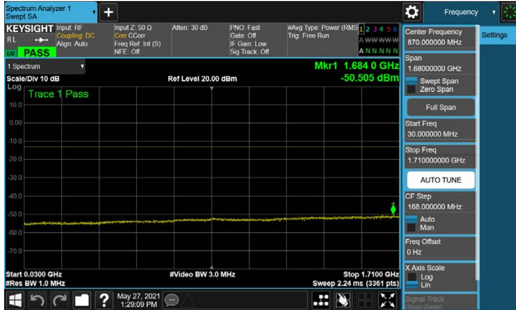
Plot 7-74. Conducted Spurious Plot (NR Band n66 - 20.0MHz - RB Size 1, RB Offset 0 - High Channel)
