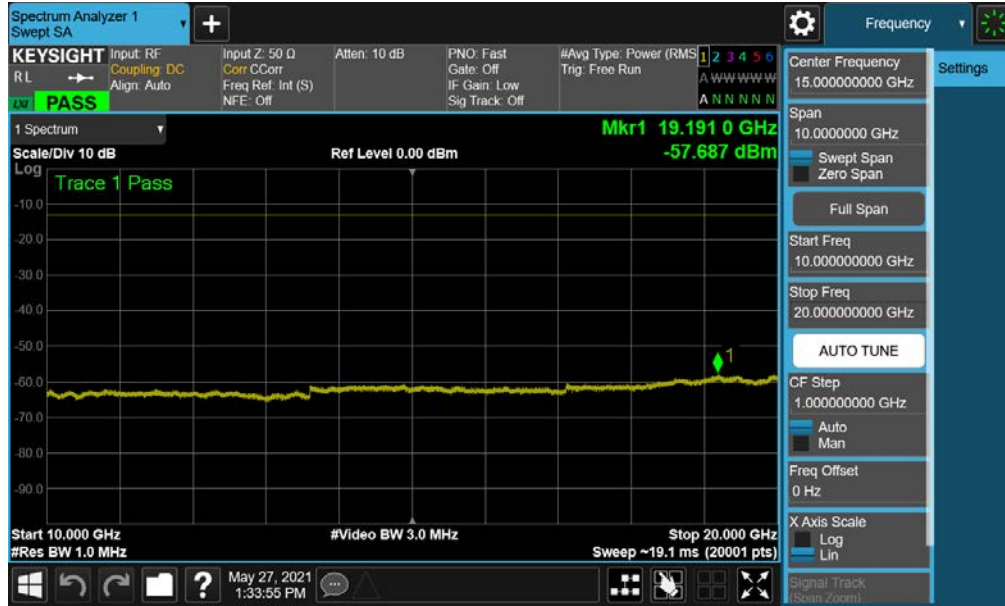
Plot 7-76. Conducted Spurious Plot (NR Band n66 - 20.0MHz - RB Size 1, RB Offset 0 - High Channel)
