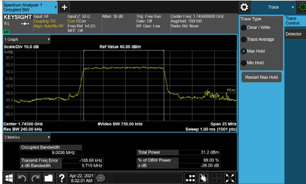
Plot 7-32. Occupied Bandwidth Plot (NR Band n66 - 10.0MHz \pi/2 BPSK - Full RB)
