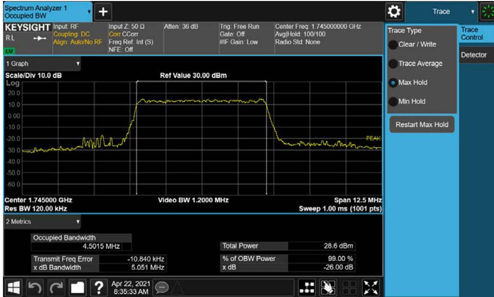
Plot 7-36. Occupied Bandwidth Plot (NR Band n66 - 5.0MHz CP-OFDM QPSK - Full RB)
