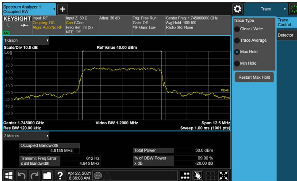
Plot 7-35. Occupied Bandwidth Plot (NR Band n66 - 5.0MHz \pi/2 BPSK - Full RB)
