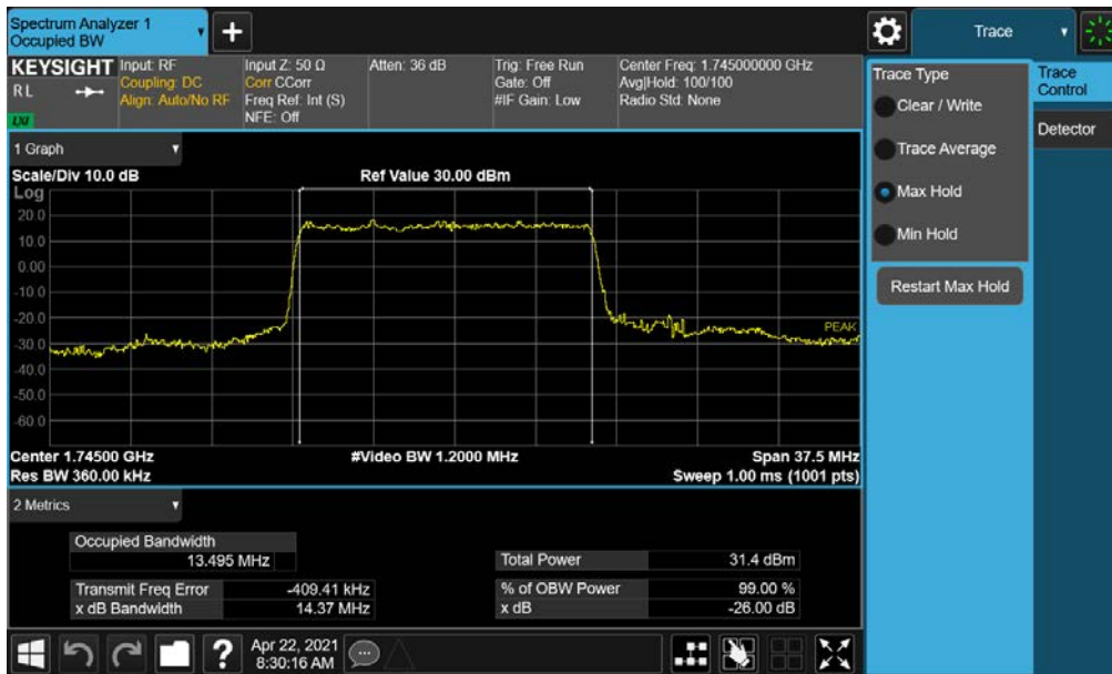
Plot 7-29. Occupied Bandwidth Plot (NR Band n66 - 15.0MHz π/2 BPSK - Full RB)
