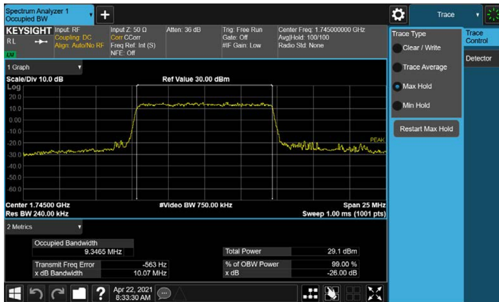
Plot 7-33. Occupied Bandwidth Plot (NR Band n66 - 10.0MHz CP-OFDM QPSK - Full RB)
