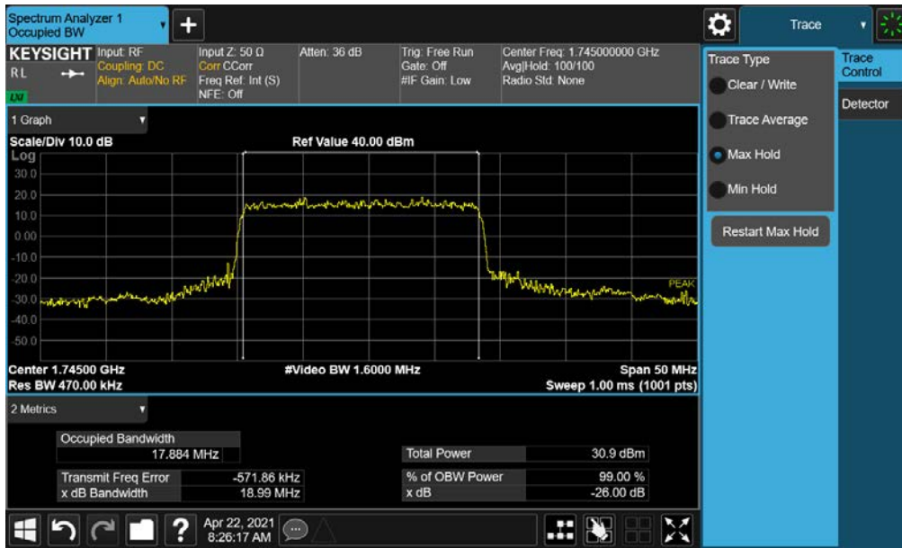
Plot 7-26. Occupied Bandwidth Plot (NR Band n66 - 20.0MHz \pi/2 BPSK - Full RB)
