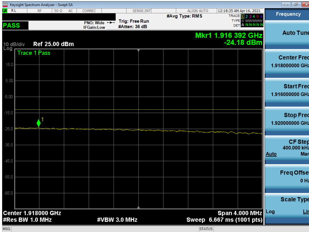
Plot 7-54. Extended Upper Band Edge Plot (LTE Band 25 - 15MHz QPSK – Full RB)
