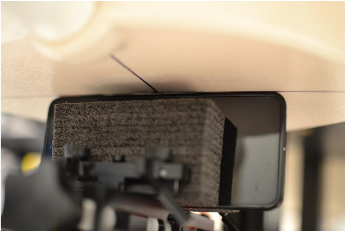
SAR Test Setup Photo 18 – Phablet, Right Edge, 0 mm
