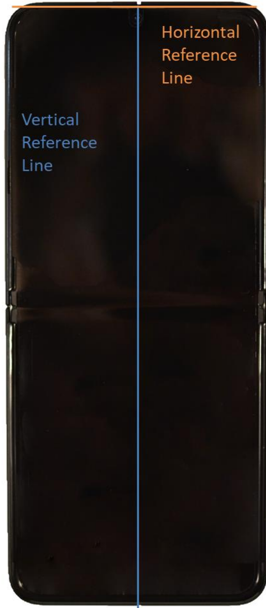
SAR Test Setup Photo 21 – Vertical and Horizontal Reference Lines
