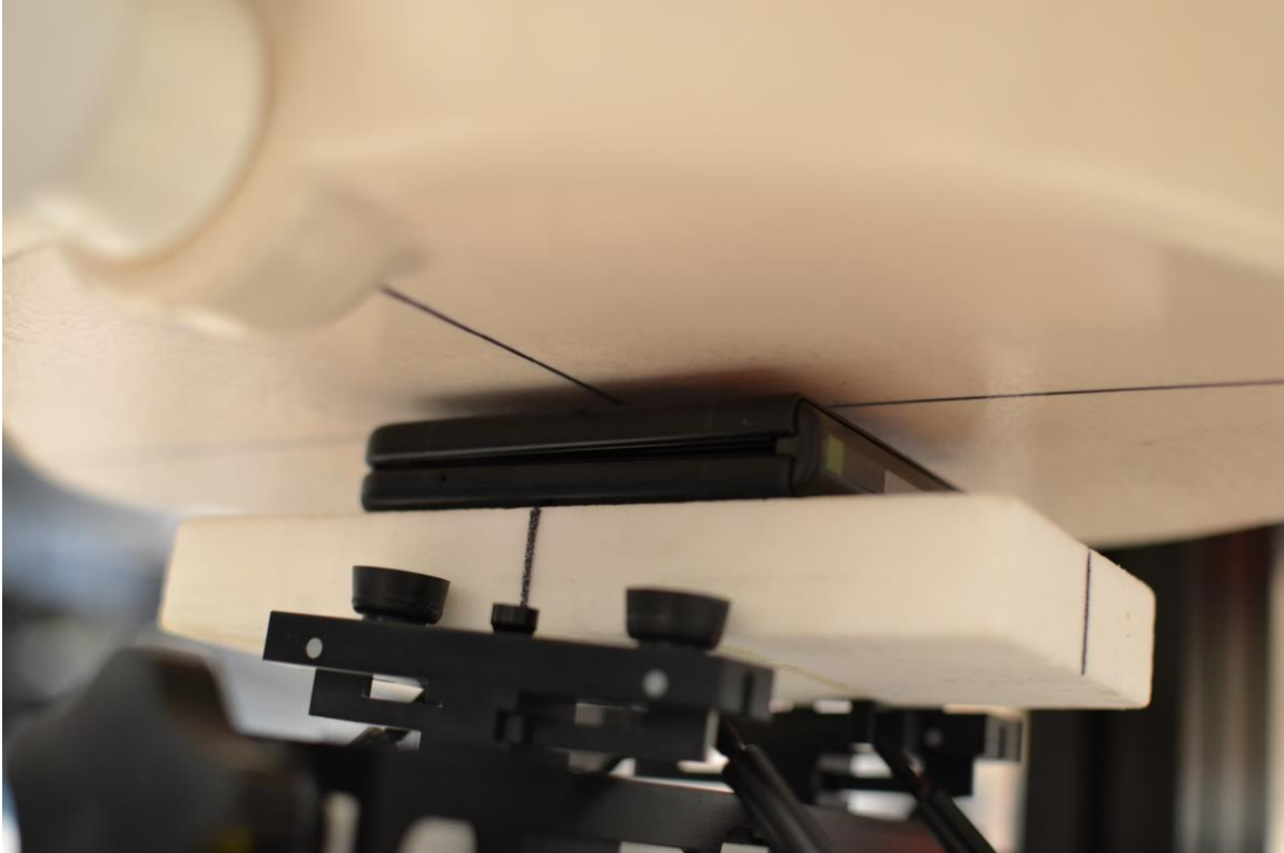
SAR Test Setup Photo 24 – Closed Hotspot, Front Side, 5 mm
