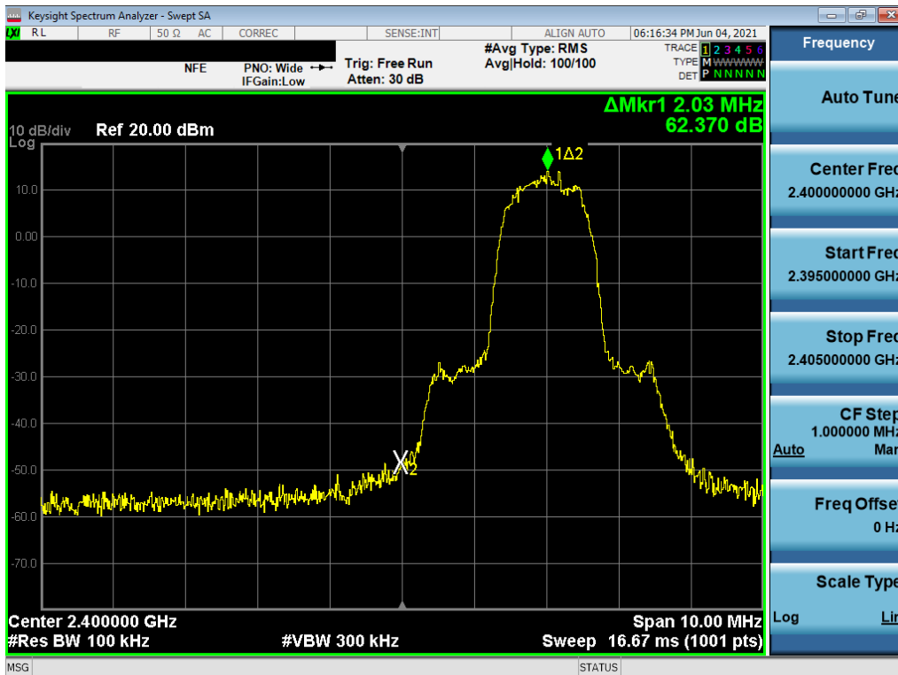
Plot 7-237. Band Edge Plot (Bluetooth with Hopping Disabled, iPA, 3 Mbps – Ch. 0) – ANT1 (N)
