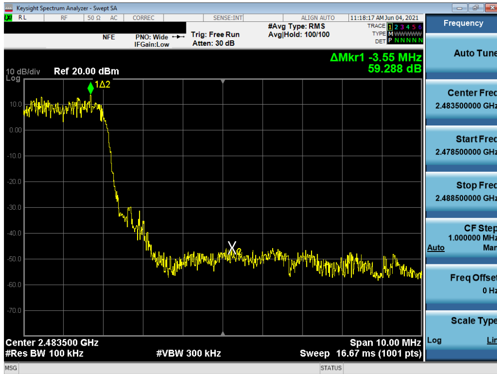
Plot 7-248. Band Edge Plot (Bluetooth with Hopping Enabled, iPA, 3 Mbps – Ch.78) – ANT1 (Q)
