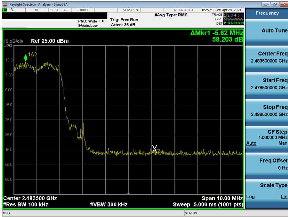
Plot 7-244. Band Edge Plot (Bluetooth with Hopping Enabled, ePA, 3 Mbps – Ch.78) – ANT1 (Q)
