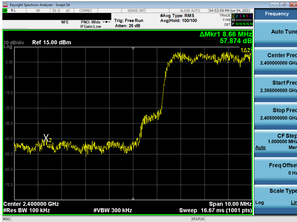
Plot 7-223. Band Edge Plot (Bluetooth with Hopping Enabled, iPA, 3 Mbps – Ch. 0) – ANT0 (N)
