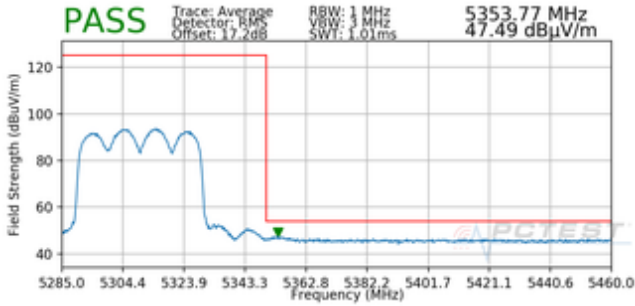
Plot 7-791. Radiated Upper Band Edge Plot MIMO with WCP (Average – UNII Band 2A)
