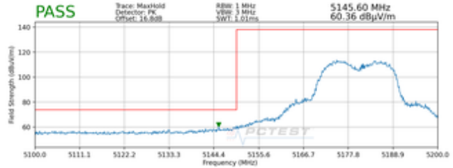
Plot 7-776. Radiated Lower Band Edge Plot MIMO (Peak – UNII Band 1)
