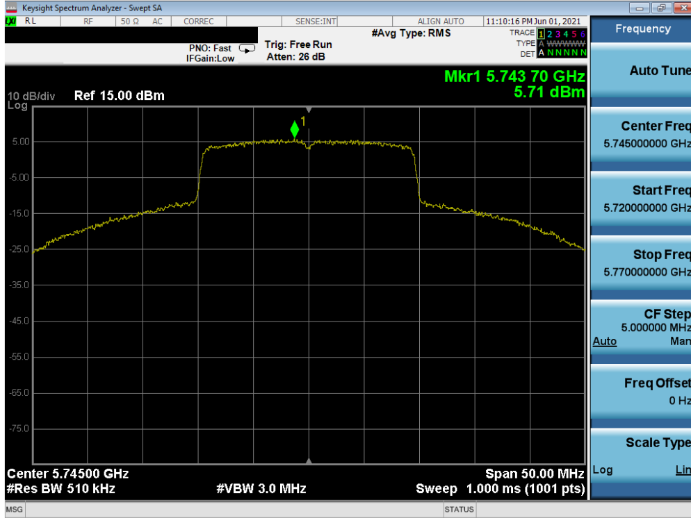
Plot 7-652. Power Spectral Density Plot MIMO ANT2 (20MHz BW 802.11ax (UNII Band 3) – Ch. 149)
