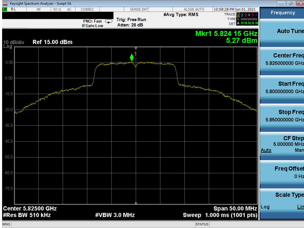
Plot 7-633. Power Spectral Density Plot MIMO ANT1 (20MHz BW 802.11a (UNII Band 3) – Ch. 165)
