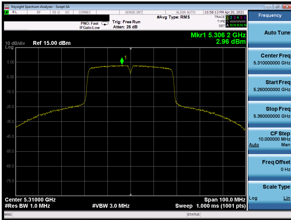
Plot 7-488. Power Spectral Density Plot SISO ANT1 (40MHz BW 802.11n (UNII Band 2A) – Ch. 62)
