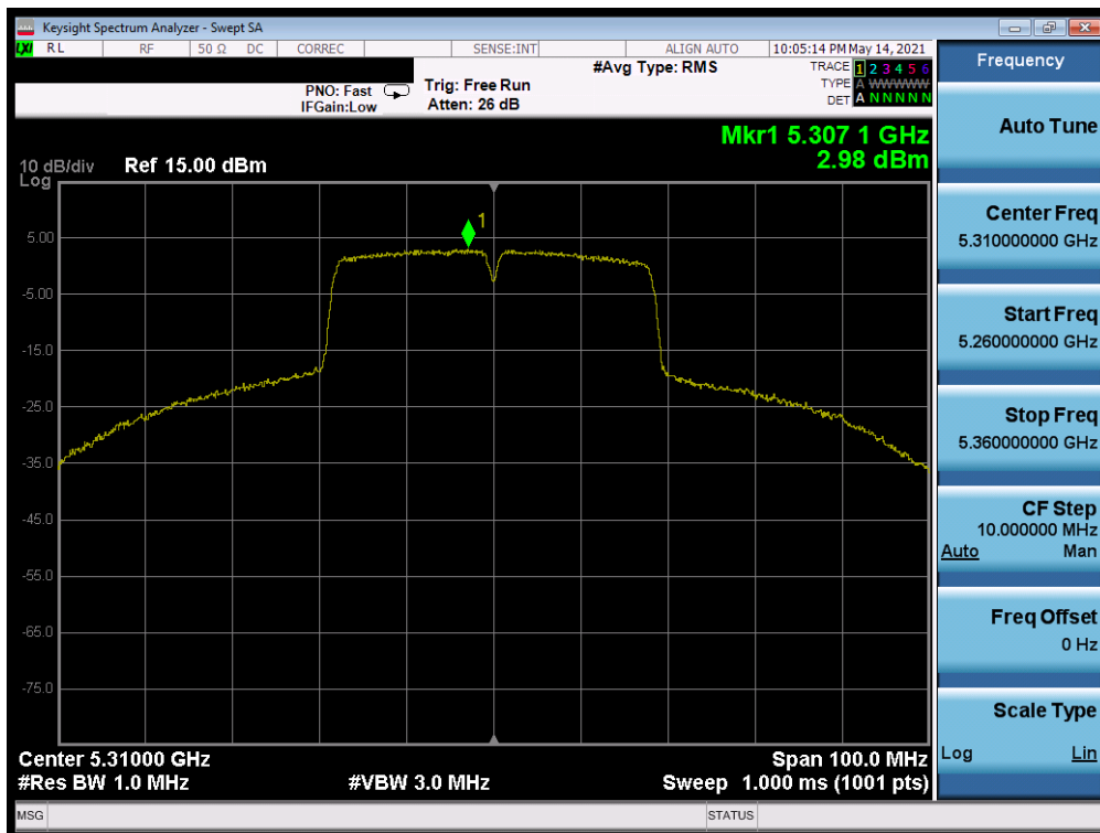
Plot 7-554. Power Spectral Density Plot MIMO ANT1 (40MHz BW 802.11n (UNII Band 2A) – Ch. 62)
