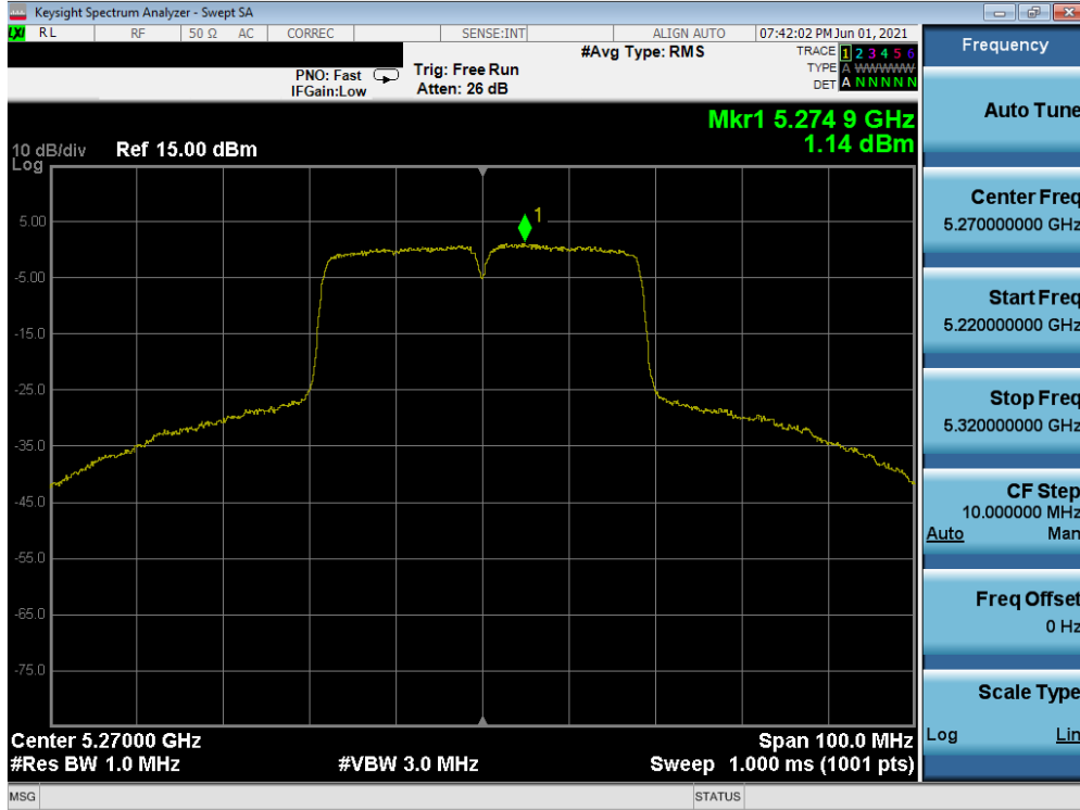
Plot 7-355. Power Spectral Density Plot MIMO ANT1 (40MHz BW 802.11n (UNII Band 2A) – Ch. 54)
