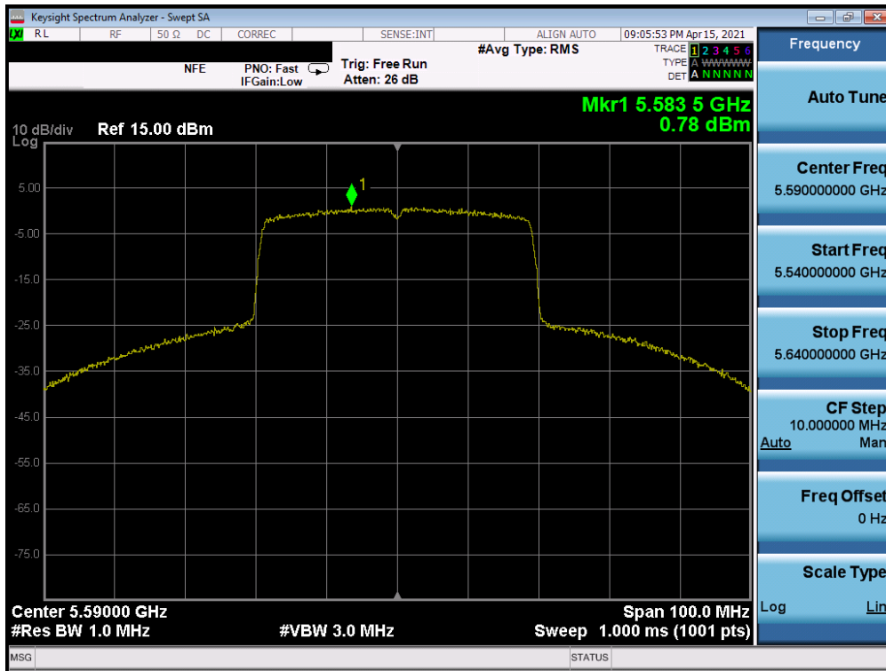
Plot 7-308. Power Spectral Density Plot SISO ANT1 (40MHz BW 802.11ax (UNII Band 2C) – Ch. 118)
