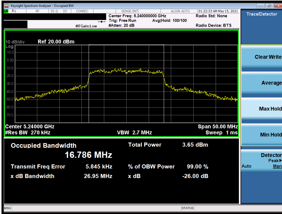
Plot 7-156. 26dB Bandwidth Plot MIMO (20MHz BW 802.11a (UNII Band 1) – Ch. 48)
