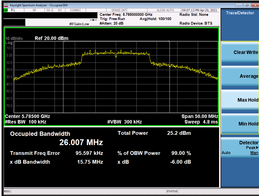
Plot 7-221. 6dB Bandwidth Plot SISO ANT1 (20MHz BW 802.11a (UNII Band 3) – Ch. 157)
