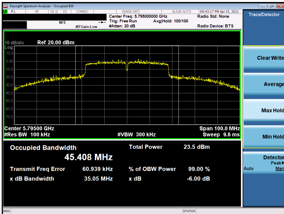
Plot 7-215. 6dB Bandwidth Plot ANT1 (40MHz BW 802.11n (UNII Band 3) – Ch. 159)
