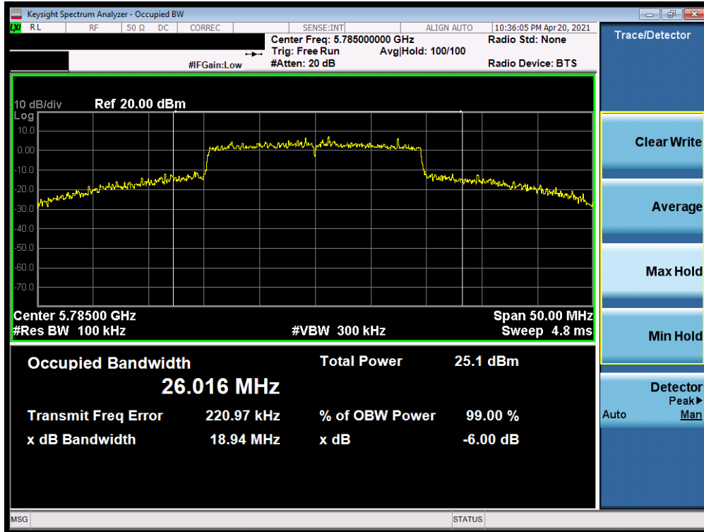
Plot 7-227. 6dB Bandwidth Plot SISO ANT1 (20MHz BW 802.11ax (UNII Band 3) – Ch. 157)
