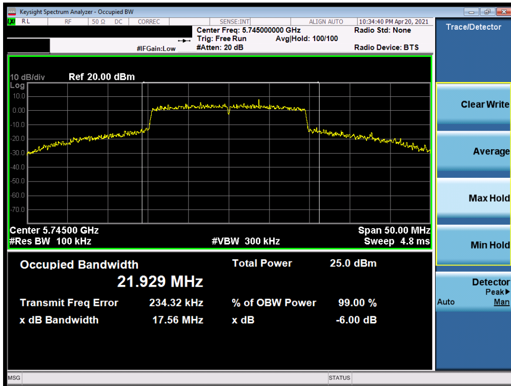
Plot 7-226. 6dB Bandwidth Plot SISO ANT1 (20MHz BW 802.11ax (UNII Band 3) – Ch. 149)
