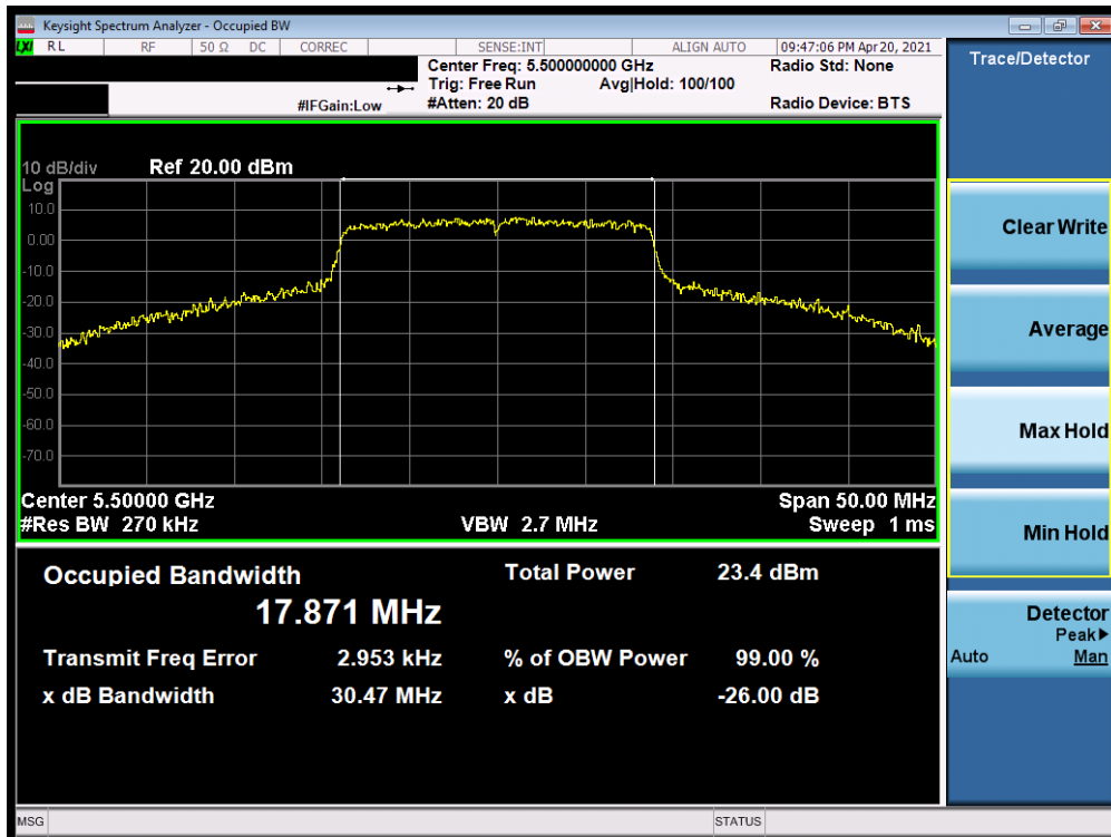
Plot 7-85. 26dB Bandwidth Plot ANT1 (20MHz BW 802.11n (UNII Band 2C) – Ch. 100)
