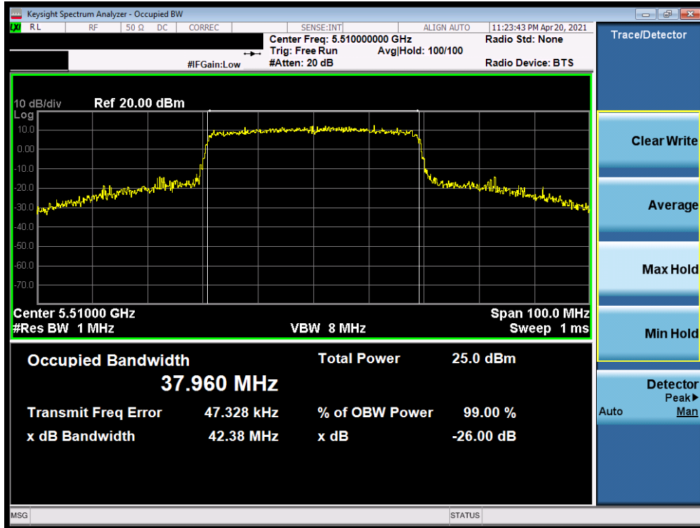
Plot 7-94. 26dB Bandwidth Plot ANT1 (40MHz BW 802.11ax (UNII Band 2C) – Ch. 102)
