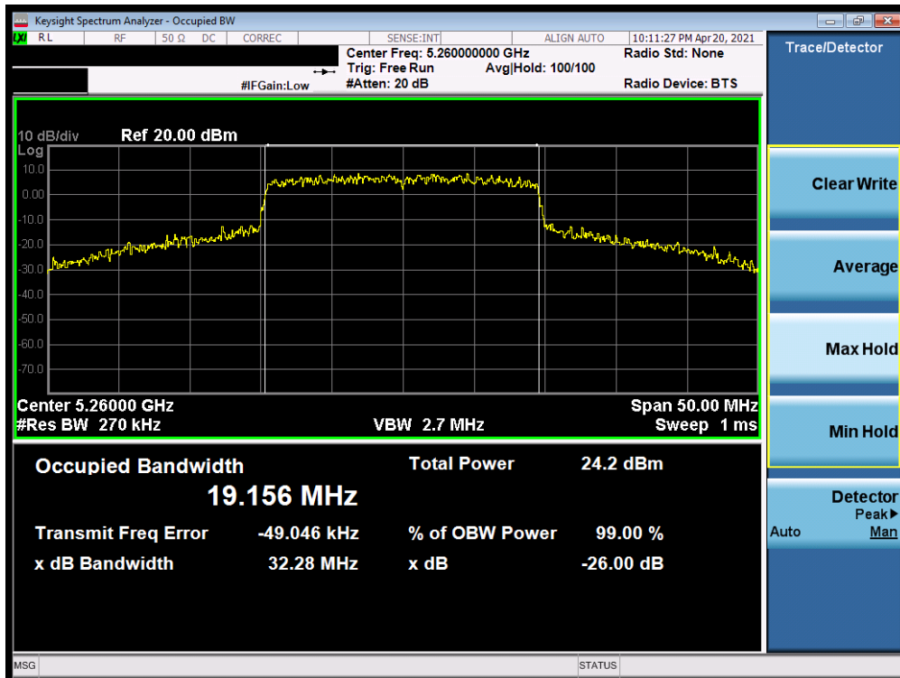
Plot 7-73. 26dB Bandwidth Plot ANT1 (20MHz BW 802.11ax (UNII Band 2A) – Ch. 52)
