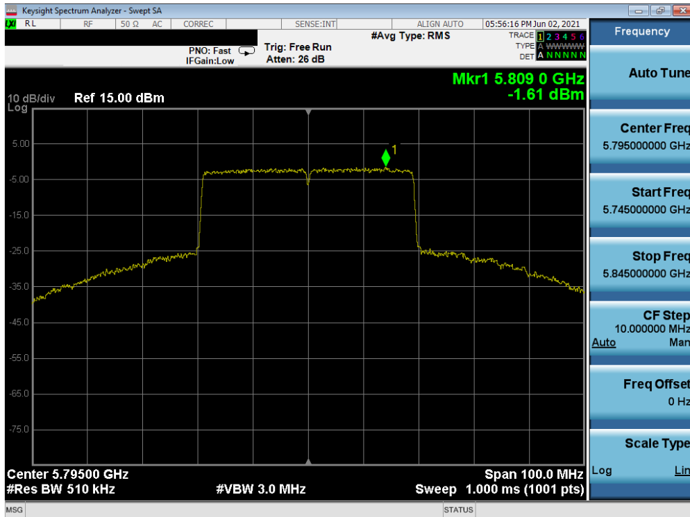
Plot 7-512. Power Spectral Density Plot MIMO ANT1 (40MHz BW 802.11ax – Full Tones (UNII Band 3) – Ch. 159)
